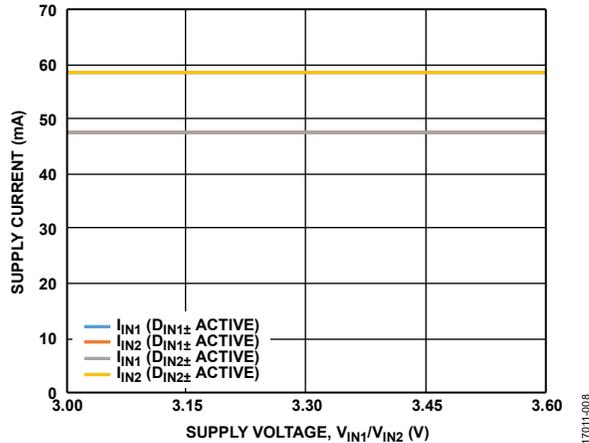
Figure 13. Supply Current vs. Supply Voltage,  $V_{IN1}/V_{IN2}$
