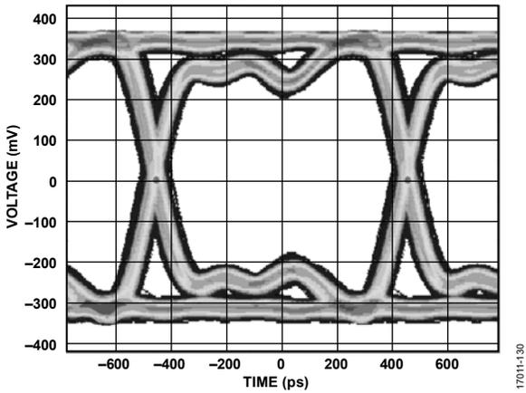
Figure 34. Eye Diagram for  $D_{OUT1\pm}$  at 550 MHz
