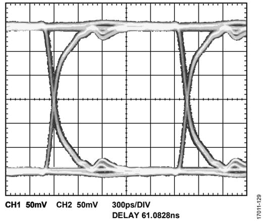
Figure 35. Eye Diagram for  $D_{OUT2\pm}$  at 300 MHz
