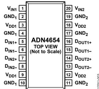
Figure 6. ADN4654 Pin Configuration
