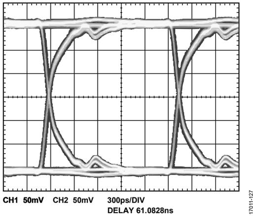
Figure 33. Eye Diagram for  $D_{OUT1\pm}$  at 300 MHz
