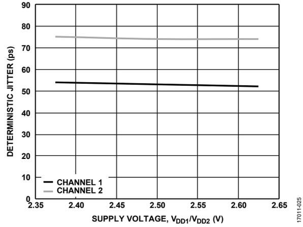
Figure 30. Deterministic Jitter vs. Supply Voltage,  $V_{DD1}/V_{DD2}$
