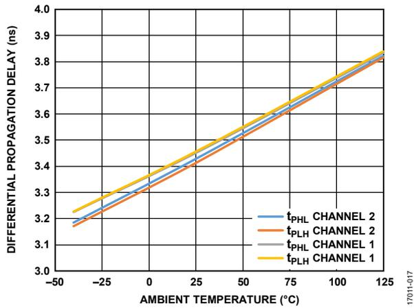
Figure 22. Differential Propagation Delay vs. Ambient Temperature
