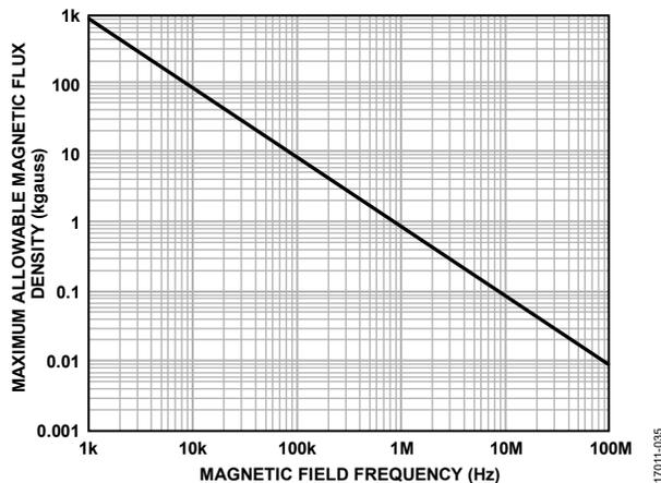
Figure 43. Maximum Allowable External Magnetic Flux Density
