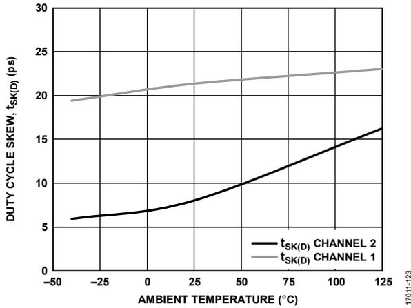
Figure 28. Duty Cycle Skew,  $t_{SK(D)}$  vs. Ambient Temperature
