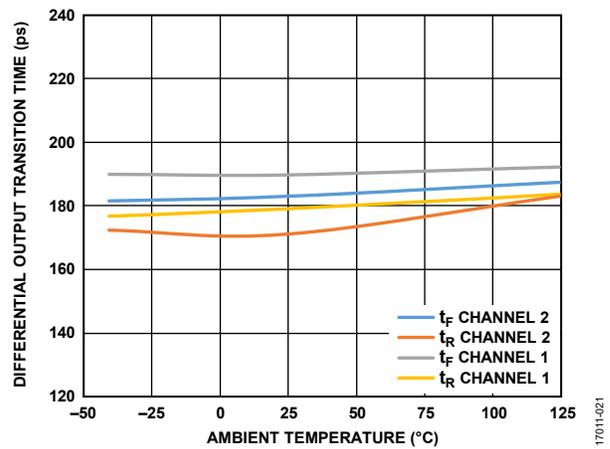
Figure 26. Differential Output Transition Time vs. Ambient Temperature
