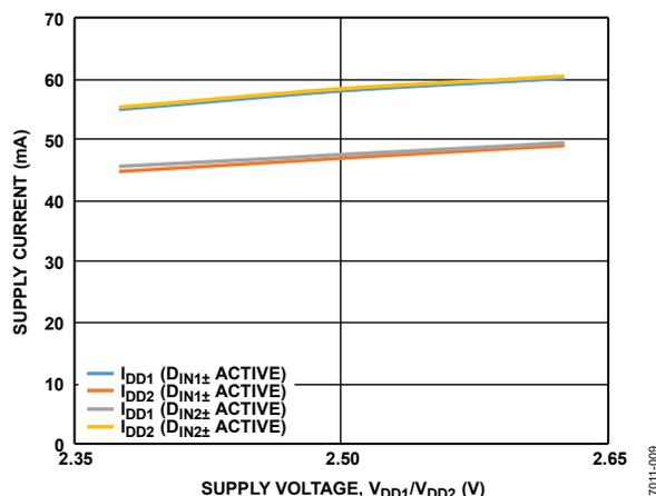
Figure 14. Supply Current vs. Supply Voltage,  $V_{DD1}/V_{DD2}$
