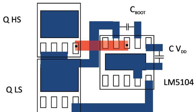
Figure 21. LM5104 Component Placement
