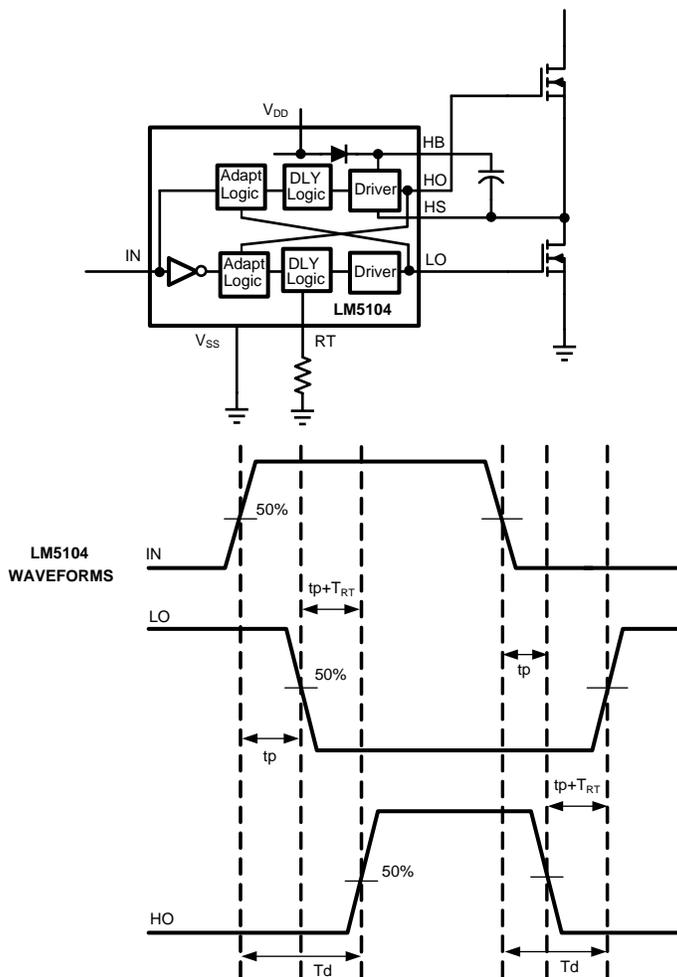
Figure 16. Application Timing Waveforms
