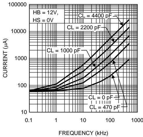
Figure 5.  $I_{HB}$  vs Frequency
