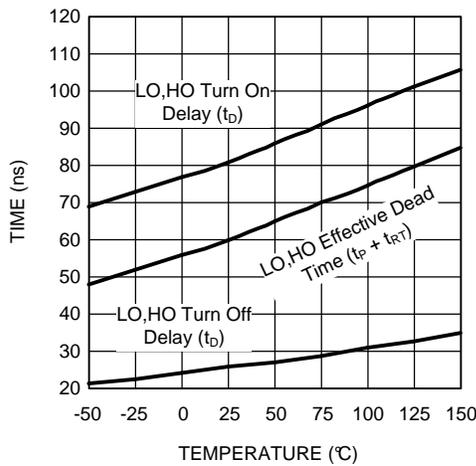
Figure 13. Timing vs Temperature RT = 10K
