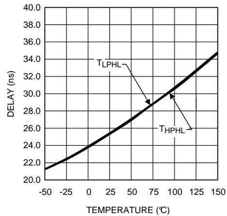
Figure 12. Turn Off Propagation Delay vs Temperature
