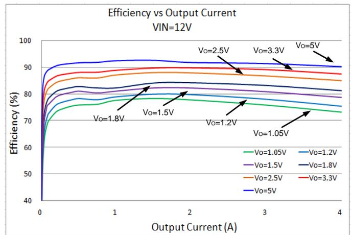
**Typical Performance Characteristics** (continued) (@ $T_A = +25^\circ\text{C}$ ,  $V_{IN} = 12\text{V}$ ,  $V_{OUT} = 1.05\text{V}$ ,  $L = 1.5\mu\text{H}$ ,  $C_1 = 20\mu\text{F}$ ,  $C_2 = 44\mu\text{F}$ , unless otherwise specified.)
