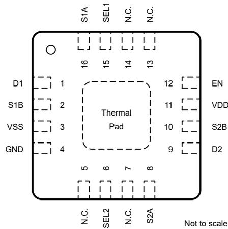
**Figure 5-1. RUM Package, 16-Pin WQFN (Top View)**
