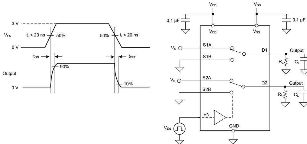
Figure 7-5. Turn-On and Turn-Off Time Measurement Setup
