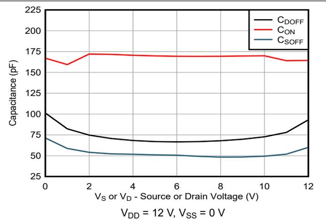
Figure 6-26. Capacitance vs Source or Drain Voltage
