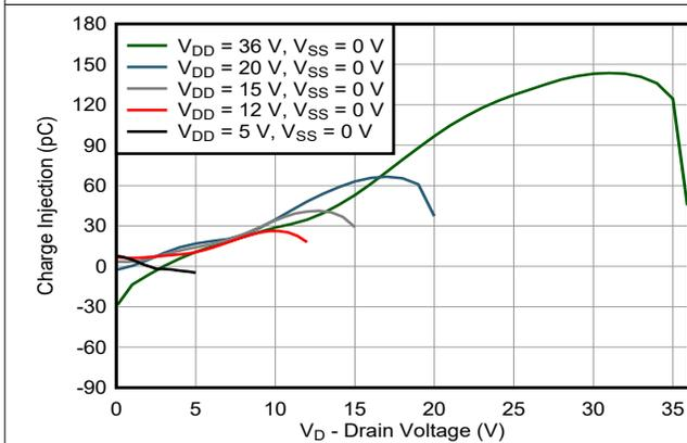
Figure 6-17. Charge Injection vs Drain Voltage – Single Supply
