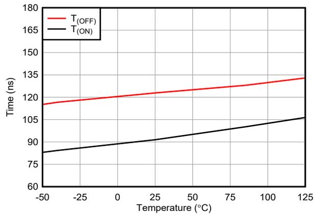
**Figure 6-21.  $T_{\text{ON}}(\text{EN})$  and  $T_{\text{OFF}}(\text{EN})$  vs Temperature**
