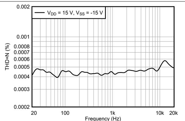
Figure 6-28. THD+N vs Frequency – Dual Supply
