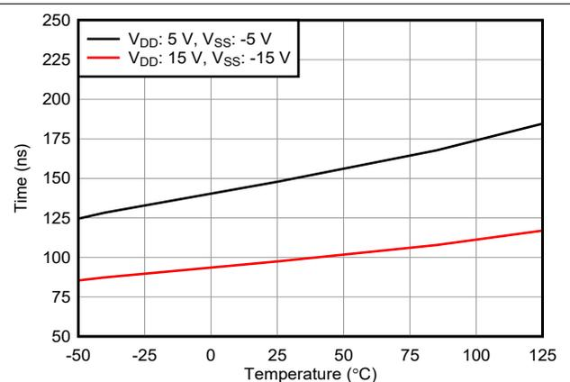
Figure 6-18.  $T_{\text{TRANSITION}}$  vs Temperature
