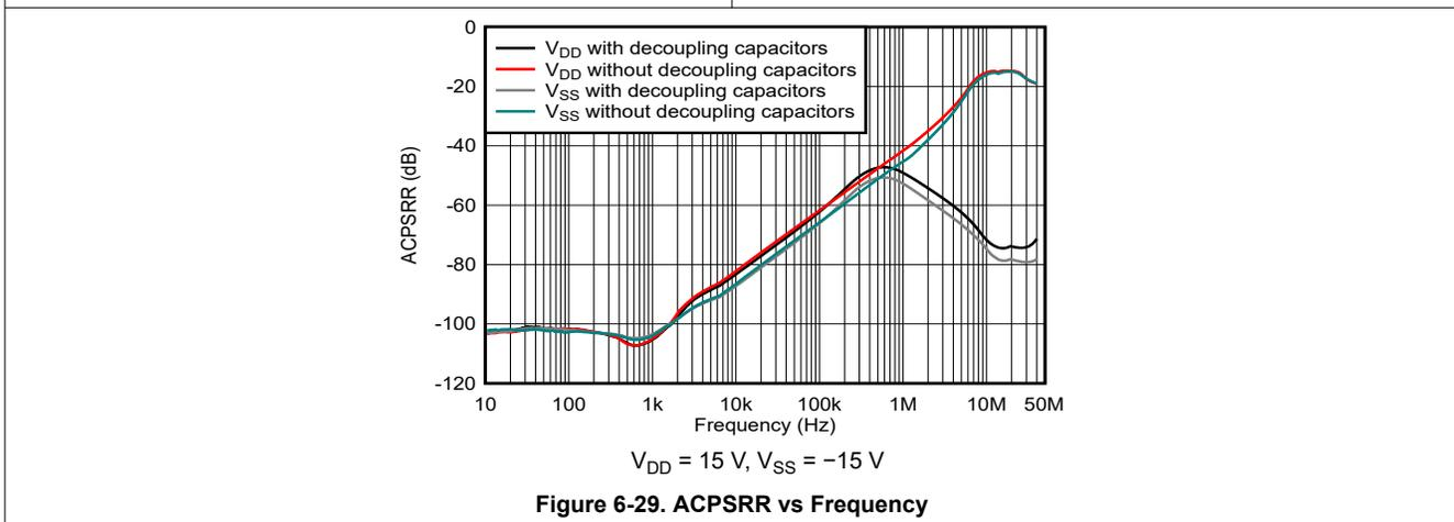
Figure 6-29. ACPSRR vs Frequency
