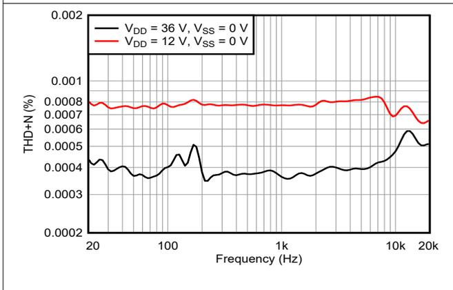
Figure 6-27. THD+N vs Frequency – Single Supply
