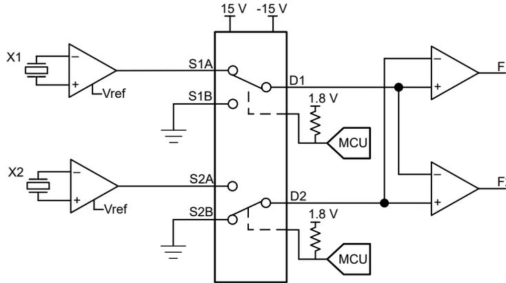
**Figure 9-1. Differential Reference Switching**
