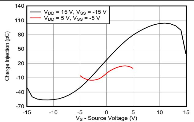
Figure 6-14. Charge Injection vs Source Voltage – Dual Supply
