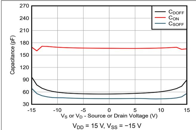
Figure 6-25. Capacitance vs Source or Drain Voltage
