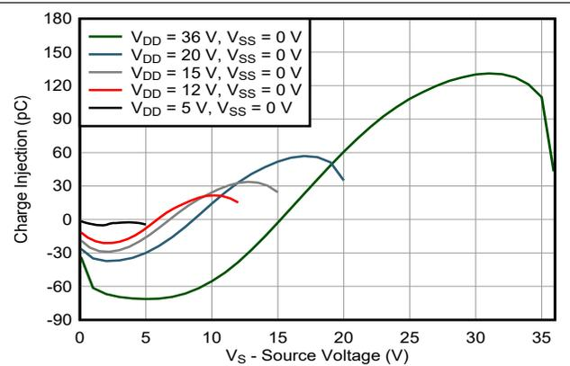
Figure 6-16. Charge Injection vs Source Voltage – Single Supply
