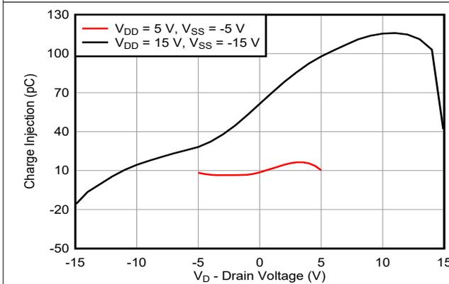
Figure 6-15. Charge Injection vs Drain Voltage – Dual Supply
