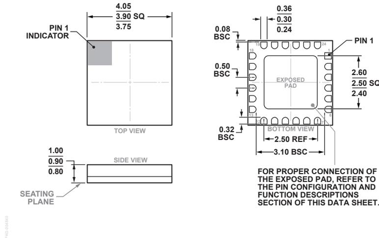
24-Terminal Ceramic Leadless Chip Carrier [LCC]
