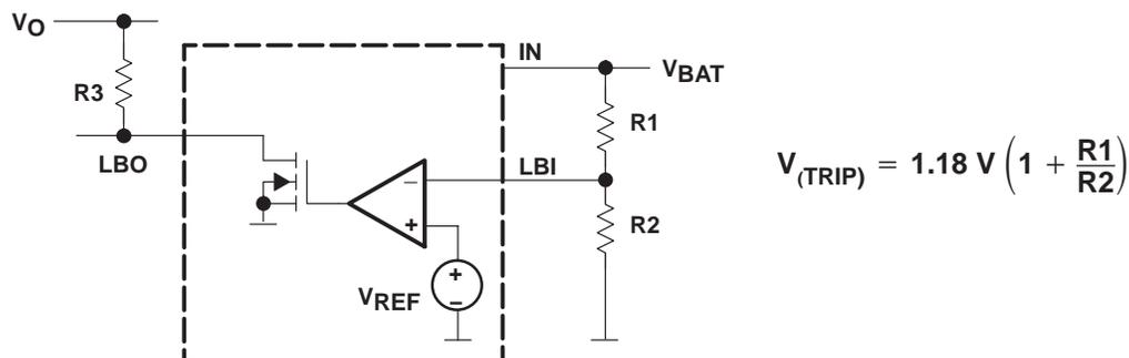
Figure 2. Programming of the Low-Battery Comparator Trip Voltage
