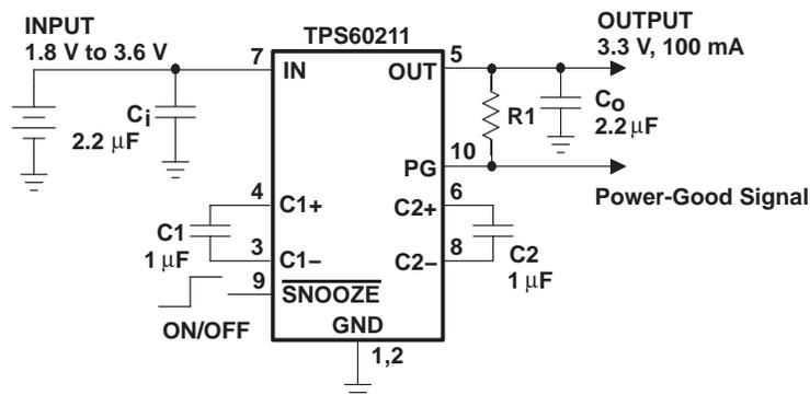
Figure 23. Typical Operating Circuit TPS60211 With Power-Good Comparator
