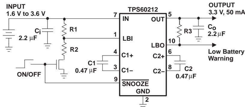
Figure 22. Typical Operating Circuit TPS60212 With Low-Battery Comparator
