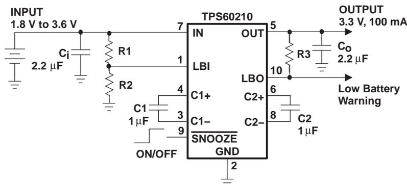
Figure 21. Typical Operating Circuit TPS60210 With Low-Battery Comparator
