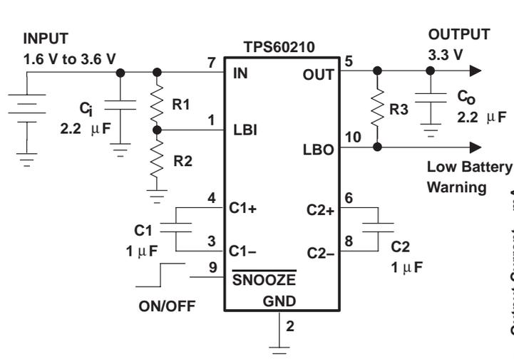
Figure 1. Typical Application Circuit With Low-Battery Warning
