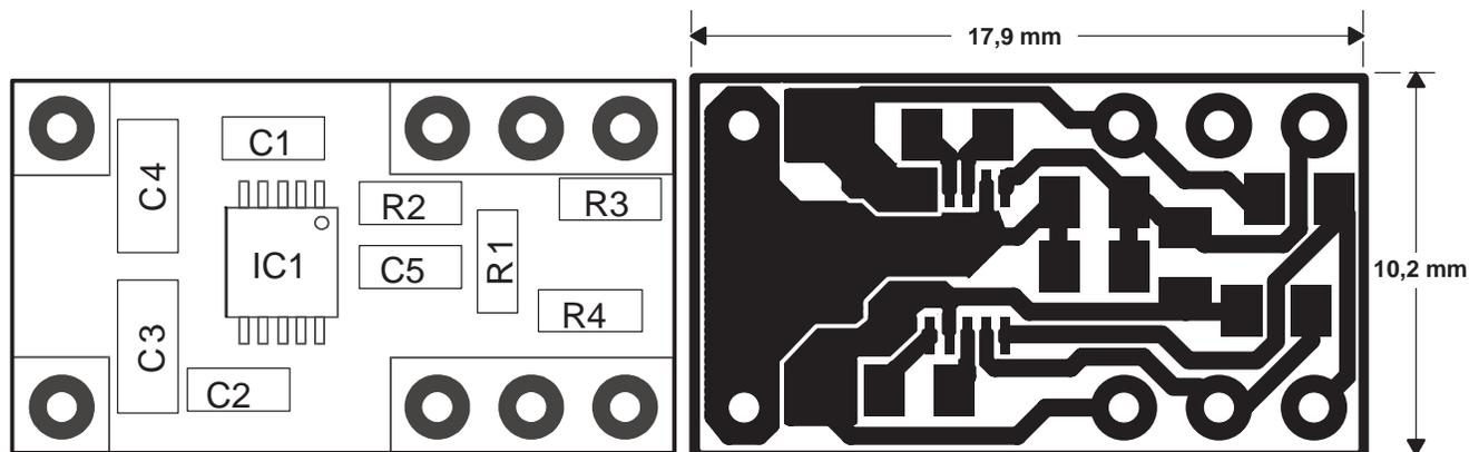
**Figure 24. Recommended Component Placement and Board Layout**
