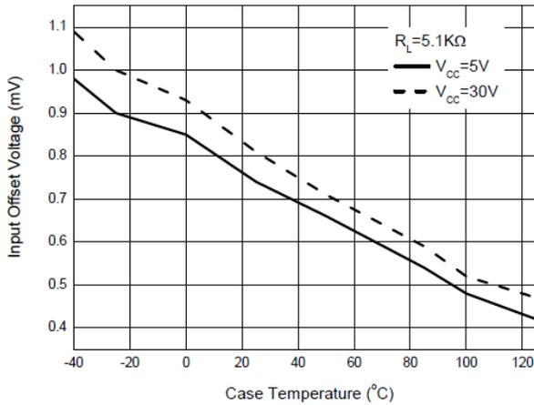
**Fig. 3 Input Offset Voltage vs. Case Temperature**
