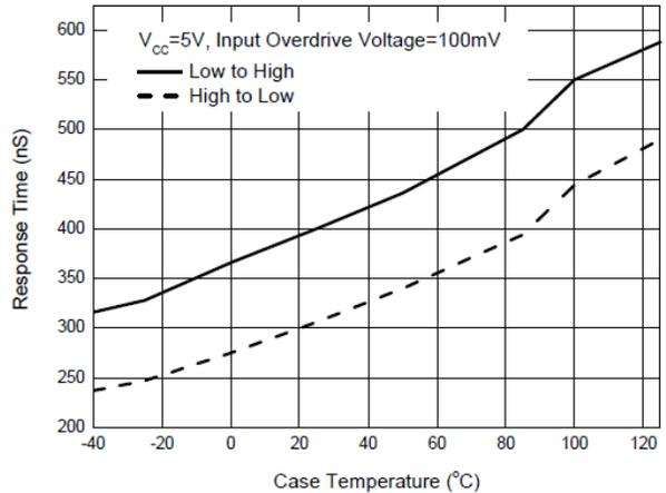
**Fig. 6 Response Time vs. Case Temperature**
