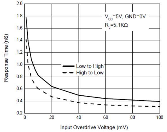
**Fig. 8 Response Time vs. Input Overdrive Voltage**
