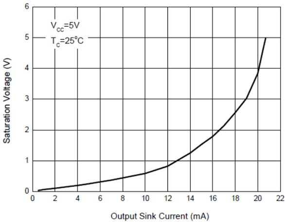
**Fig. 5 Saturation Voltage vs. Output Sink Current**
