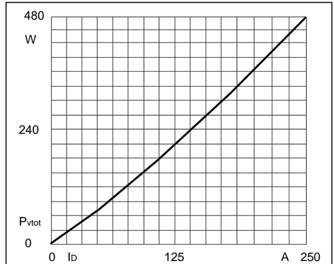
Fig2. Power dissipation
