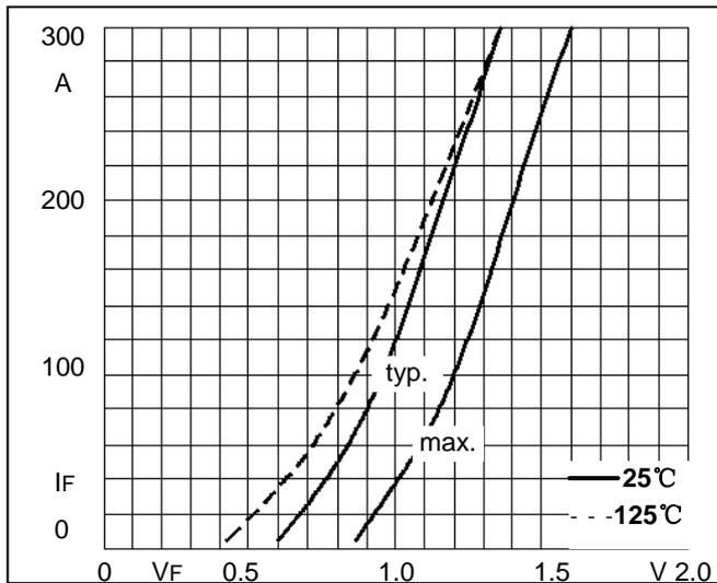
Fig1. Forward Characteristics
