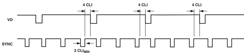
Figure 17. Example of Synchronization with SYNCPOL = 0 and SYNCCNT = 3
