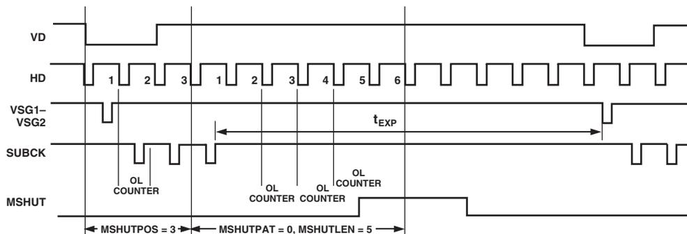
Figure 46. Example of MSHUT High Precision Timing—MSHUTEN = 1 and MSHUTPOS\_HP = 3
