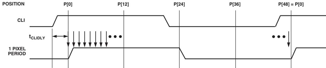
1. PIXEL CLOCK PERIOD IS DIVIDED INTO 48 POSITIONS, PROVIDING FINE EDGE RESOLUTION FOR HIGH SPEED CLOCKS.
