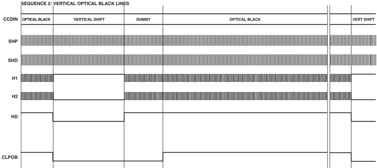
Figure 56. Horizontal Sequence during Vertical Optical Black Pixels
