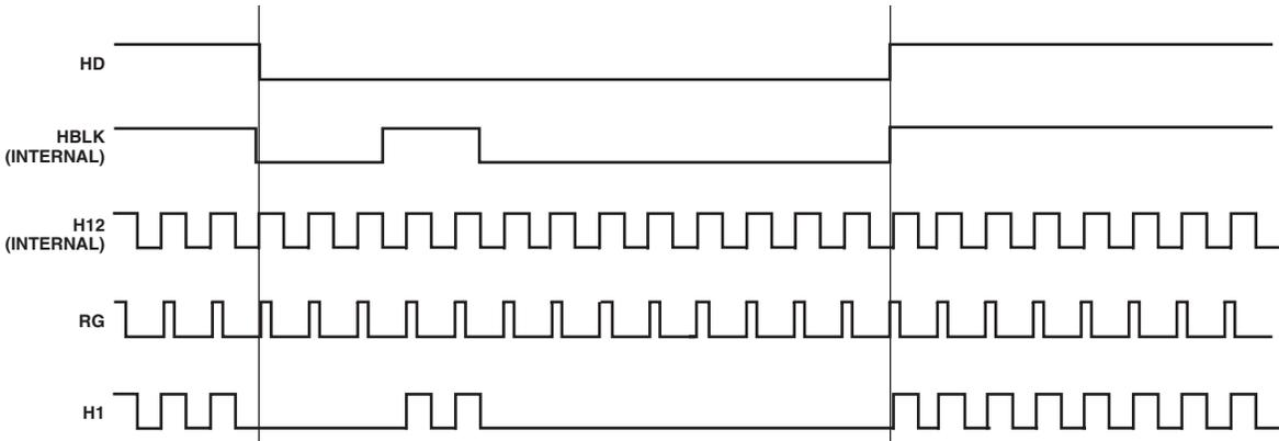
Figure 24. Selective H-Blanking Operation  $HBLKMASK = 0$ ,  $HPULSECNT = 1$ ,  $HBLKHPOS = 003$
