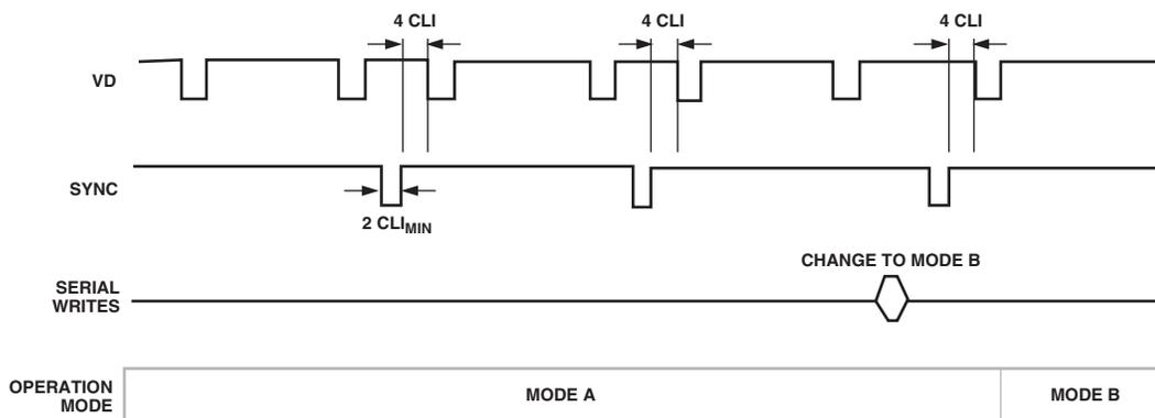
Figure 16. Example of Synchronization with SYNCPOL = 0 and SYNCCNT = 1
