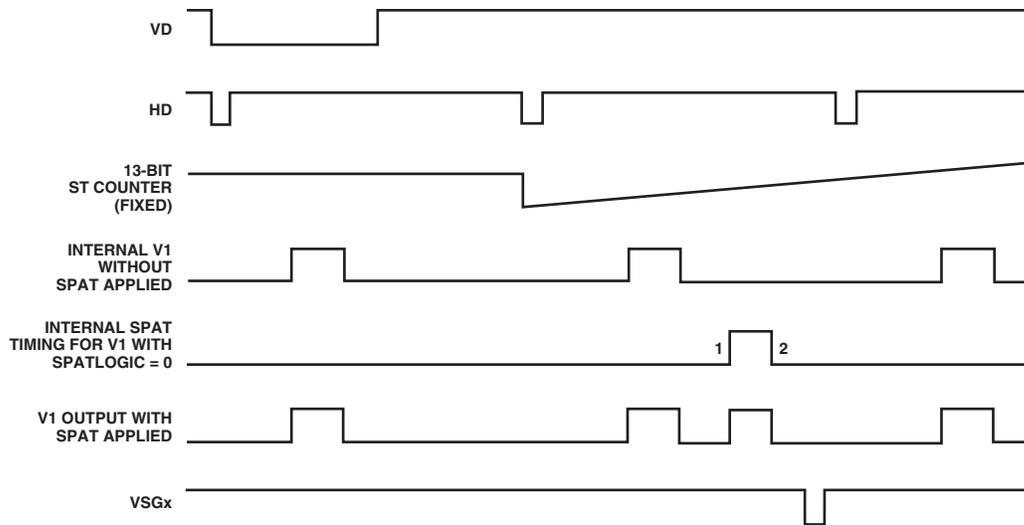
1. THE  $VxSPAT\_TOG1$  AND  $VxSPAT\_TOG2$  REGISTERS REFERENCE THE 13-BIT ST COUNTER.
