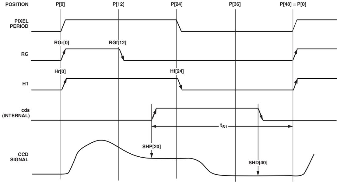
1. ALL SIGNAL EDGES ARE FULLY PROGRAMMABLE TO ANY OF THE 48 POSITIONS WITHIN ONE PIXEL PERIOD.
