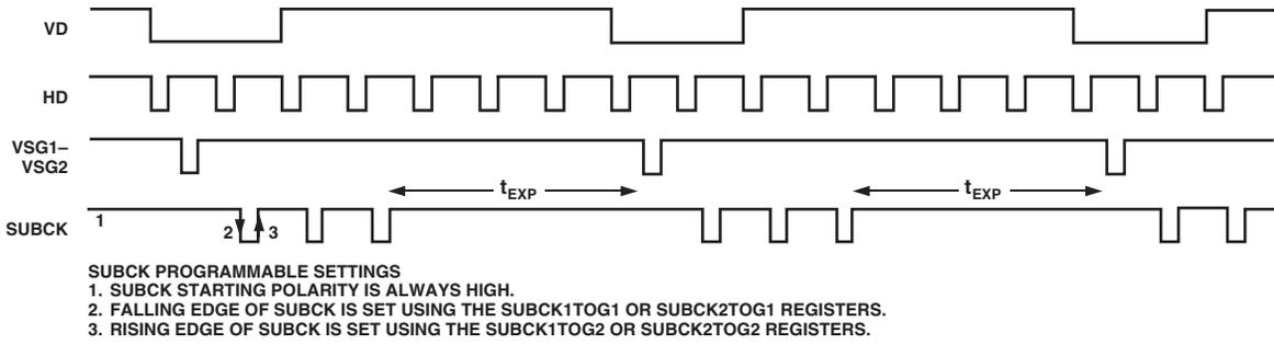
NUMBER OF SUBCK PULSES WITHIN THE FIELD IS SET USING THE SUBCKNUM REGISTER. IN THIS EXAMPLE, SUBCKNUM = 2.
