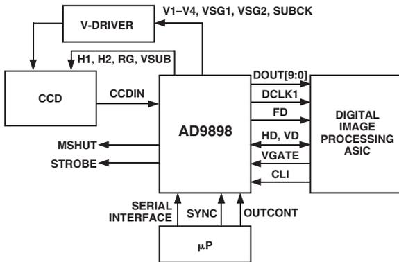
Figure 5. Typical System Block Diagram, Master Mode
