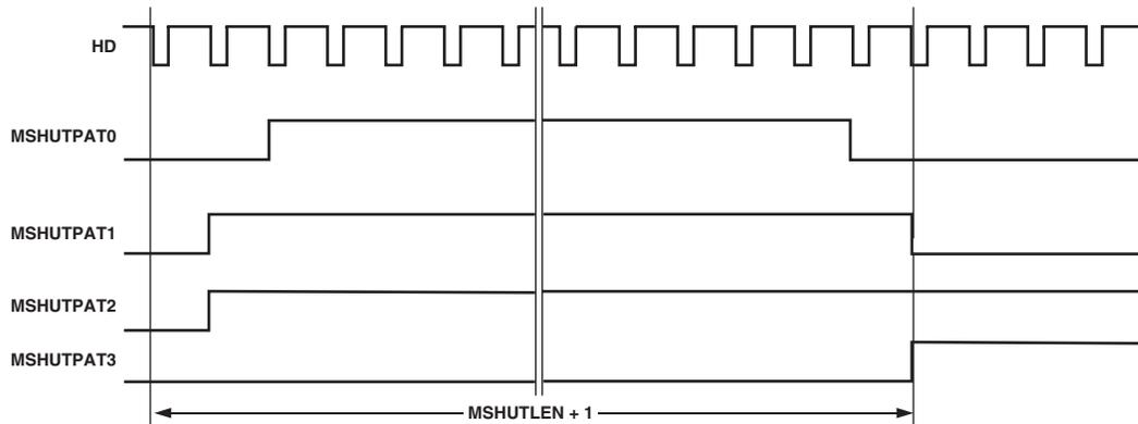
*Figure 44. MSHUT Patterns Available by Setting MSHUTPAT Register*
