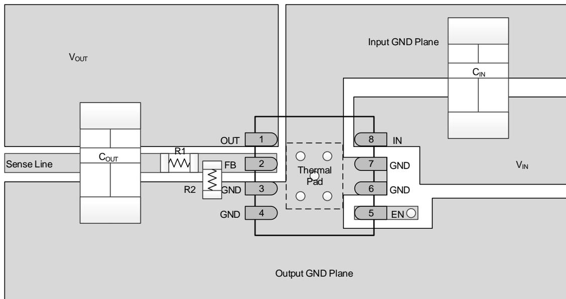
NOTE:  $C_{IN}$  and  $C_{OUT}$  are size 1208 capacitors, while  $R_1$  and  $R_2$  are size 0402.
