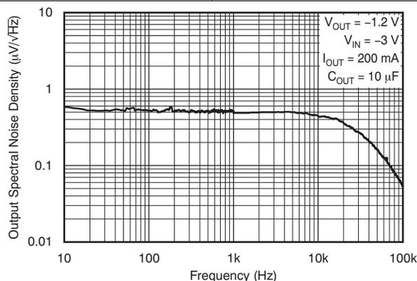
Figure 17. Output Spectral Noise Density
