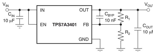
**Figure 19. Adjustable Operation for Maximum AC Performance**
