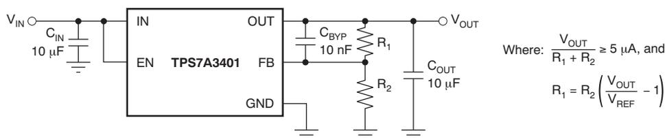
Figure 21. Maximize PSRR Performance and Minimize RMS Noise
