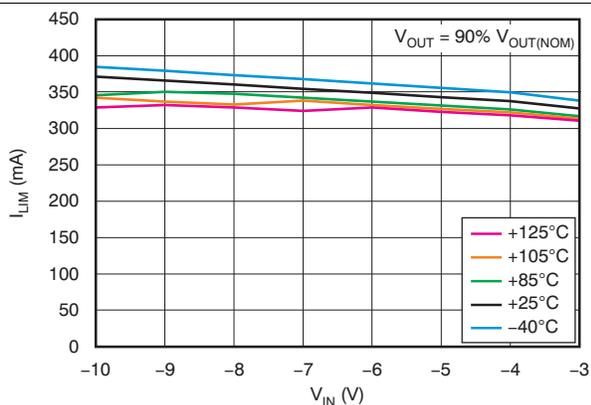
**Figure 11. Current Limit vs Input Voltage**
