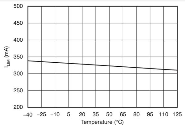
**Figure 12. Current Limit vs Temperature**
