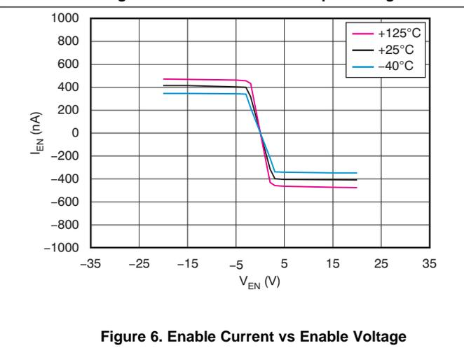
Figure 6. Enable Current vs Enable Voltage
