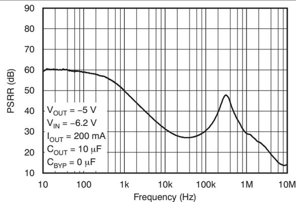
Figure 15. Power-Supply Rejection Ratio
