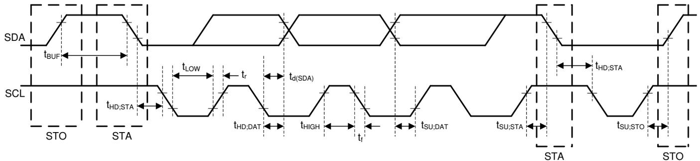
Figure 7-1. I<sup>2</sup>C Interface Timing Diagram
