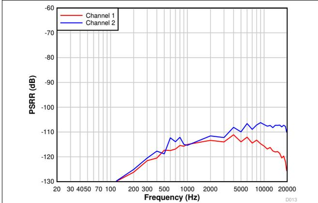
**Figure 7-16. Power-Supply Rejection Ratio vs Ripple Frequency With 100-mV<sub>pp</sub> Amplitude**
