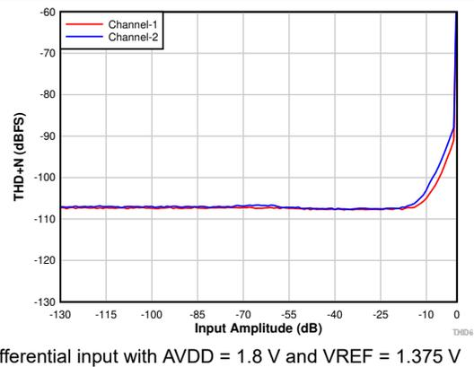
Differential input with  $AVDD = 1.8\text{ V}$  and  $VREF = 1.375\text{ V}$
