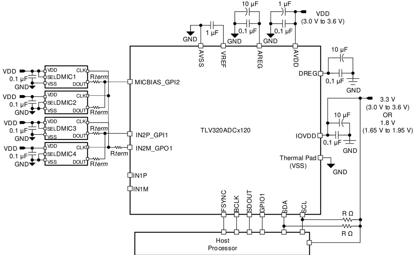
Figure 9-6. Four-Channel Digital PDM Microphone Recording Diagram
