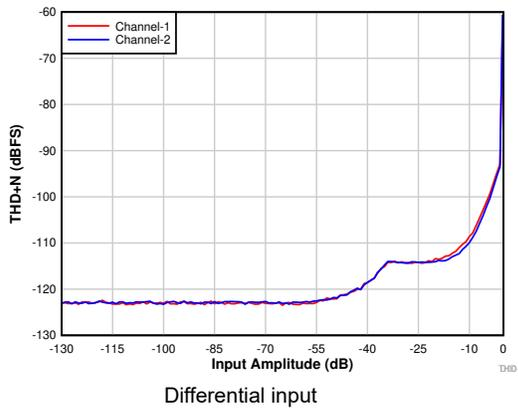
**Figure 7-4. THD+N vs Input Amplitude With DRE Enabled**
