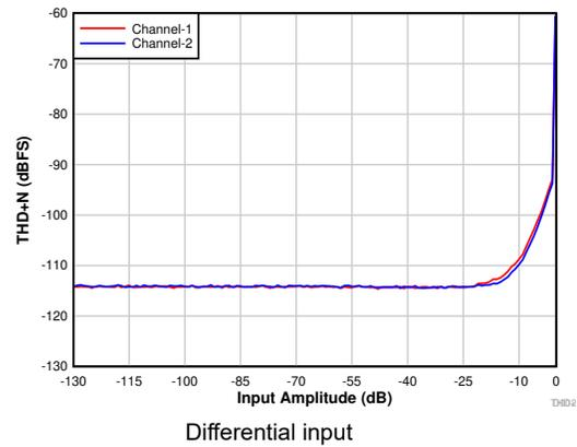
**Figure 7-5. THD+N vs Input Amplitude With DRE Disabled**
