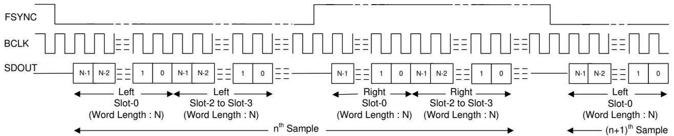
**Figure 8-8. I²S Protocol Timing (TX\_OFFSET = 0 and BCLK\_POL = 1)**
