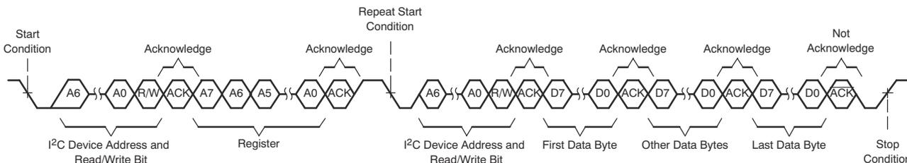
**Figure 8-70. I<sup>2</sup>C Multiple-Byte Read Transfer**
