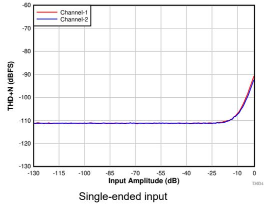
**Figure 7-7. THD+N vs Input Amplitude With DRE Disabled**
