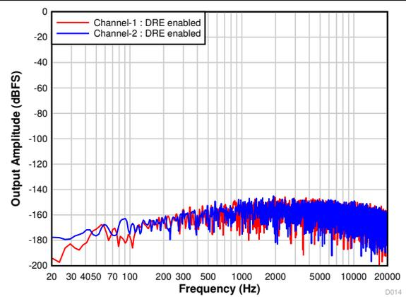
**Figure 7-17. FFT With Idle Input With DRE Enabled**
