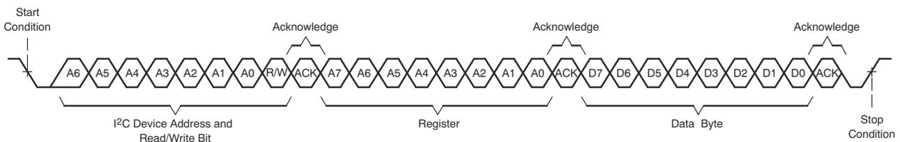
**Figure 8-67. I<sup>2</sup>C Single-Byte Write Transfer**
