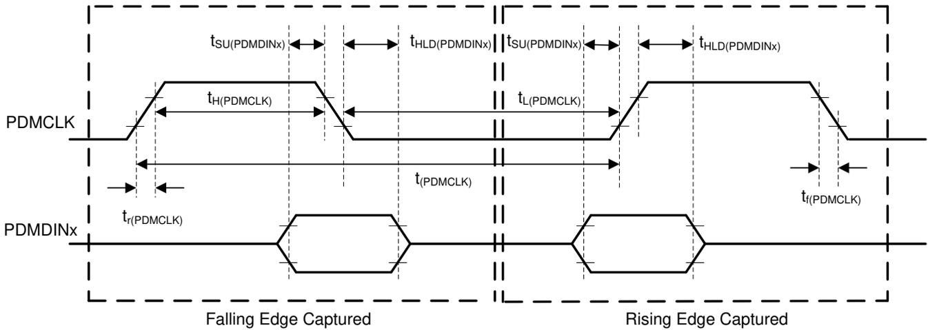
**Figure 7-3. PDM Digital Microphone Interface Timing Diagram**
