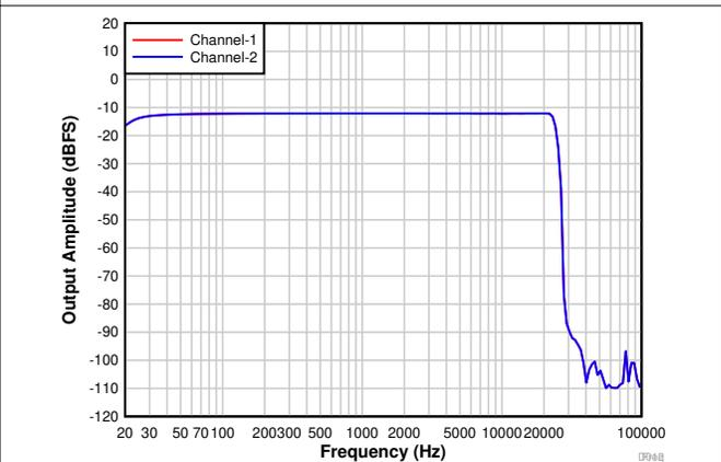
Figure 7-15. Frequency Response With a -12-dBr Input
