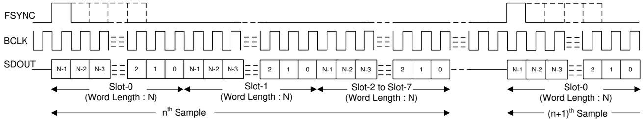
Figure 8-4. TDM Mode Protocol Timing (TX\_OFFSET = 0 and BCLK\_POL = 1)
