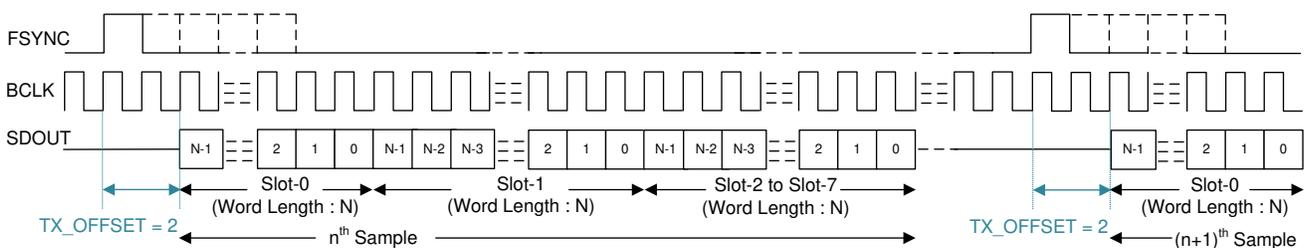
**Figure 8-2. TDM Mode Protocol Timing (TX\_OFFSET = 2)**
