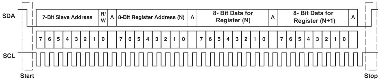
**Figure 8-66. Typical I<sup>2</sup>C Sequence**
