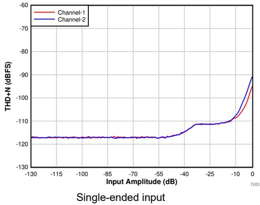
**Figure 7-6. THD+N vs Input Amplitude With DRE Enabled**
