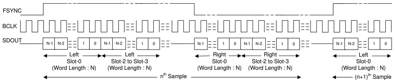
**Figure 8-9. LJ Mode Standard Protocol Timing (TX\_OFFSET = 0)**
