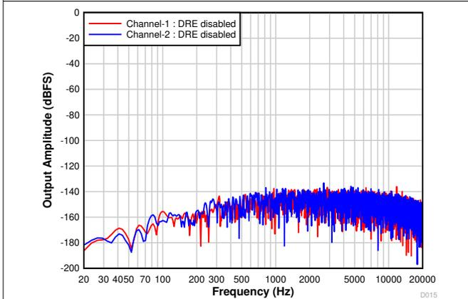
**Figure 7-18. FFT With Idle Input With DRE Disabled**
