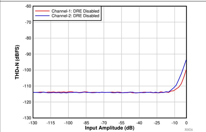
**Figure 9-5. THD+N vs Input Amplitude With DRE Disabled**
