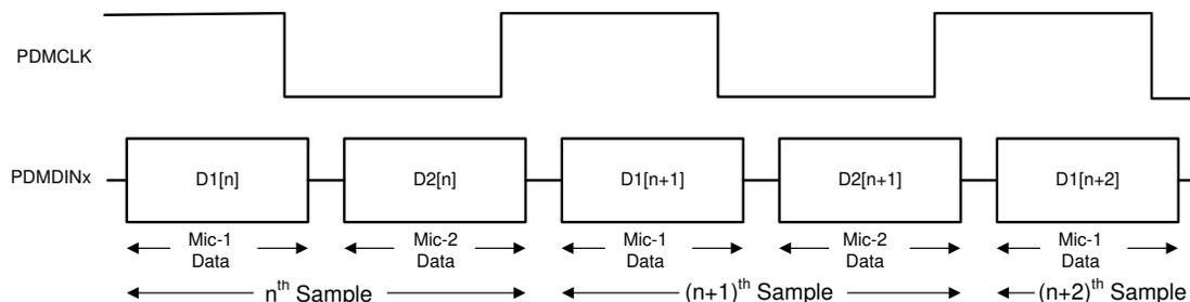
**Figure 8-65. Digital PDM Microphone Protocol Timing Diagram**
