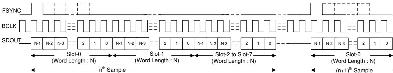
**Figure 8-1. TDM Mode Standard Protocol Timing (TX\_OFFSET = 0)**
