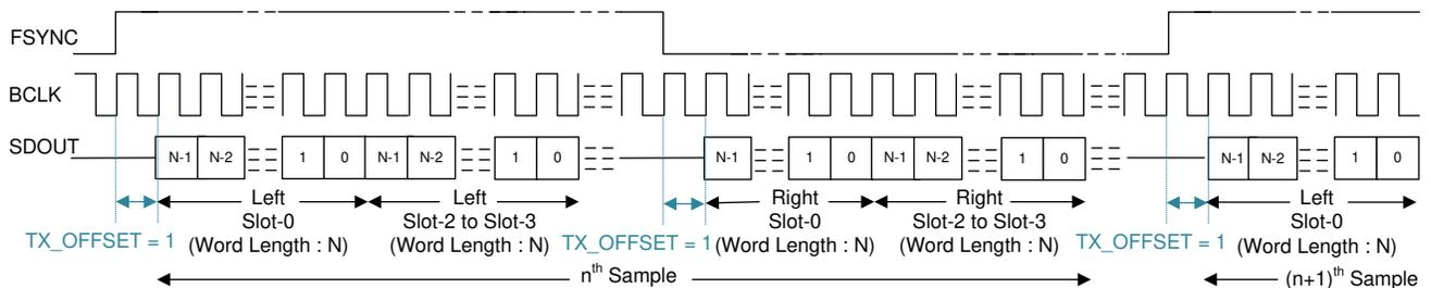
Figure 8-12. LJ Protocol Timing (TX\_OFFSET = 1 and BCLK\_POL = 1)
