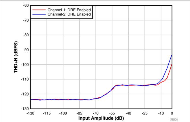
**Figure 9-3. THD+N vs Input Amplitude With DRE Enabled**
