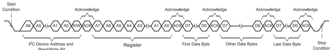
**Figure 8-68. I<sup>2</sup>C Multiple-Byte Write Transfer**
