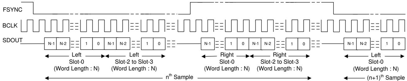
Figure 8-5. I<sup>2</sup>S Mode Standard Protocol Timing (TX\_OFFSET = 0)
