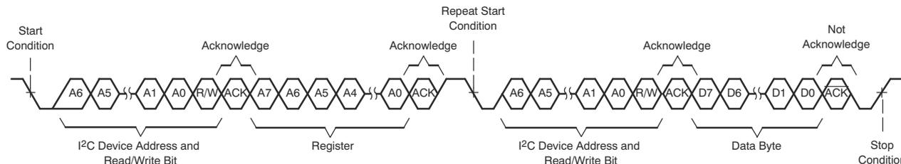
**Figure 8-69. I<sup>2</sup>C Single-Byte Read Transfer**
