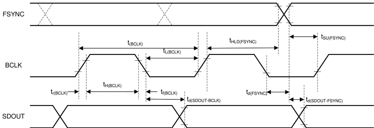
Figure 7-2. TDM (With BCLK\_POL = 1), I<sup>2</sup>S, and LJ Interface Timing Diagram
