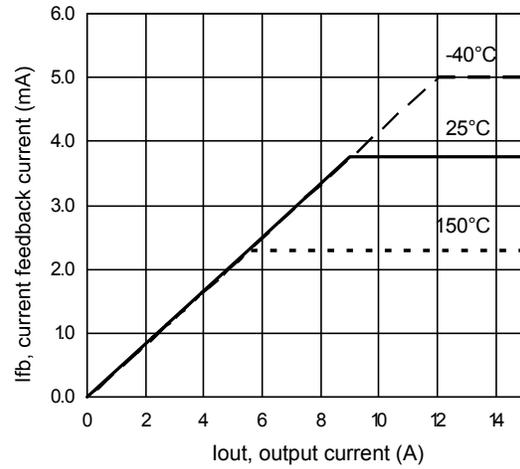
**Figure 10 – I<sub>fb</sub> (mA) Vs I<sub>out</sub> (A)**
