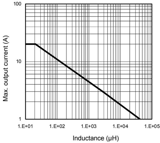
**Figure 9 – Max. I<sub>out</sub> (A) Vs inductance (µH)**
