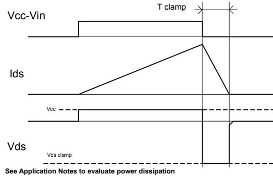
**Figure 2 – Active clamp waveforms**
