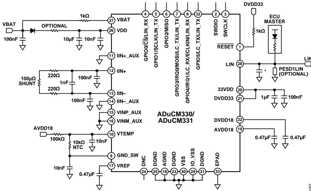
\*LIN 2.2 PHYSICAL TEST PASSED WITH 220pF CAPACITOR.
