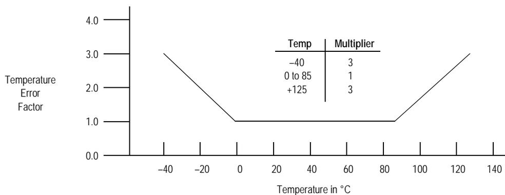
NOTE: The Temperature Multiplier is a linear response from 0° to -40°C and from 85° to 125°C.
