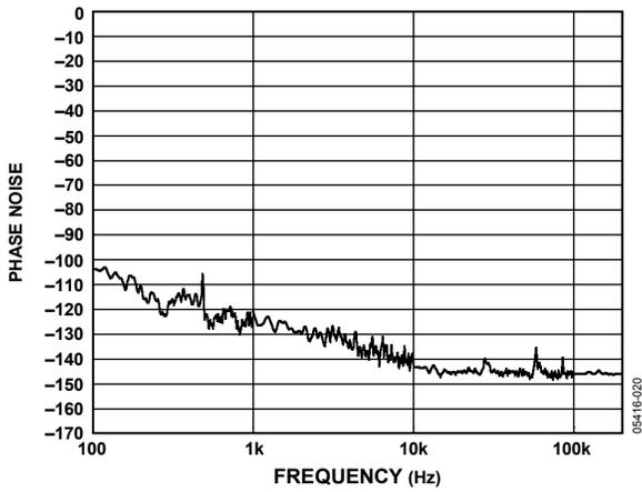
Figure 20. Output Phase Noise
