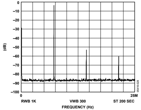
Figure 28.  $f_{MCLK} = 50 \text{ MHz}$ ,  $f_{OUT} = 7.143 \text{ MHz} = f_{MCLK}/7$ ,
