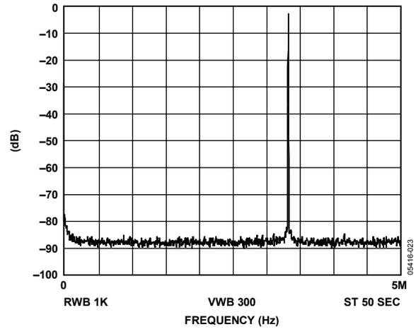
Figure 23.  $f_{MCLK} = 10 \text{ MHz}$ ,  $f_{OUT} = 3.33 \text{ MHz} = f_{MCLK}/3$ ,
