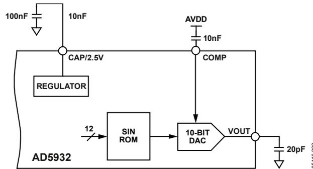
Figure 2. Test Circuit Used to Test the Specifications
