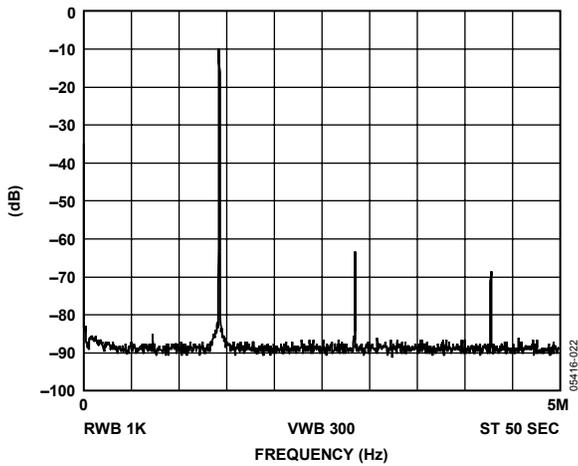
Figure 22.  $f_{MCLK} = 10 \text{ MHz}$ ,  $f_{OUT} = 1.43 \text{ MHz} = f_{MCLK}/7$ ,
