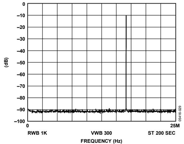
Figure 29.  $f_{MCLK} = 50 \text{ MHz}$ ,  $f_{OUT} = 16.667 \text{ MHz} = f_{MCLK}/3$ ,
