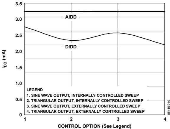
Figure 10.  $I_{DD}$  vs. Output Waveform Type and Control
