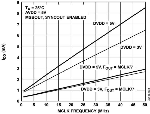
Figure 8. Current Consumption ( $I_{DD}$ ) vs. MCLK Frequency
