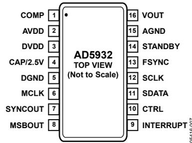
Figure 7. Pin Configuration
