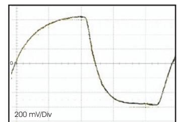
Note: The clipped sinewave output is AC coupled
