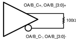
**Figure 7-3. DS90C189-Q1 (Transmitter) LVDS Output Load**
