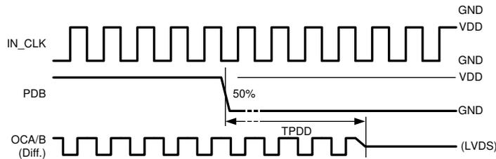
**Figure 7-8. Sleep Mode / Power Down Delay**
