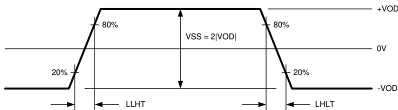
**Figure 7-4. LVDS Output Transition Times**
