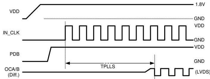
**Figure 7-7. Start Up / Phase Lock Loop Set Time**
