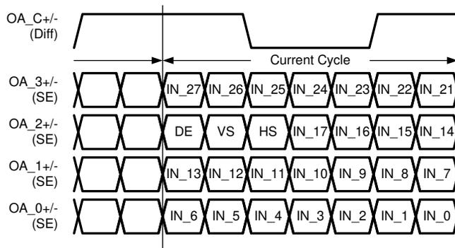
**Figure 8-2. Single Pixel / 24bpp LVDS Mapping**
