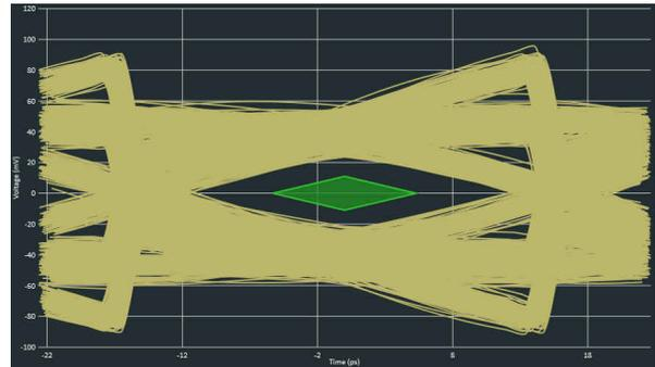
**Figure 8-8. PCIe 5.0 Link Setup with the DS320PR810 Eye Diagram Using SigTest**
