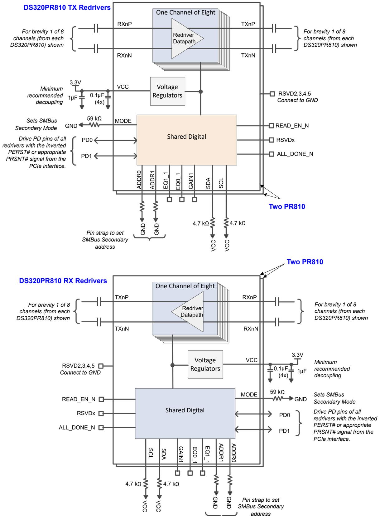
Figure 8-4. Simplified Schematic for PCIe x16 Lane Configuration in SMBus/I<sup>2</sup>C Secondary mode
