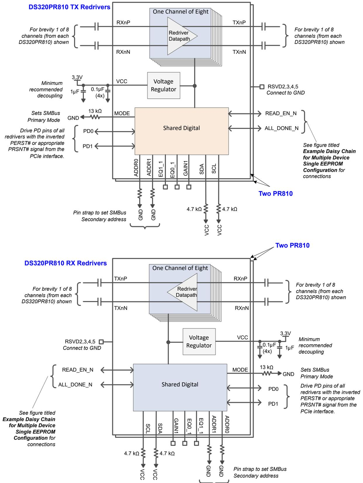
Figure 8-3. Simplified Schematic for PCIe x16 Lane Configuration in SMBus/I<sup>2</sup>C Primary mode
