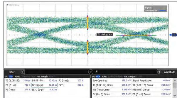
Figure 6-5. Through Baseline Calibration Trace Setup (7 dB Loss)
