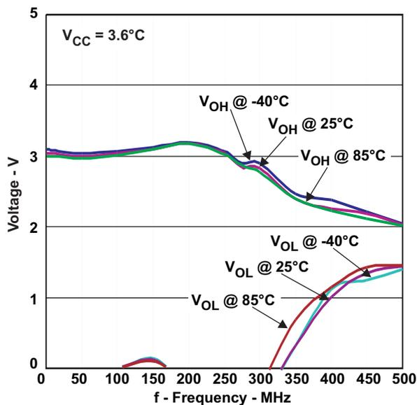
Figure 3. Maximum Switching Frequency  $V_{CC} = 3.6 V$
