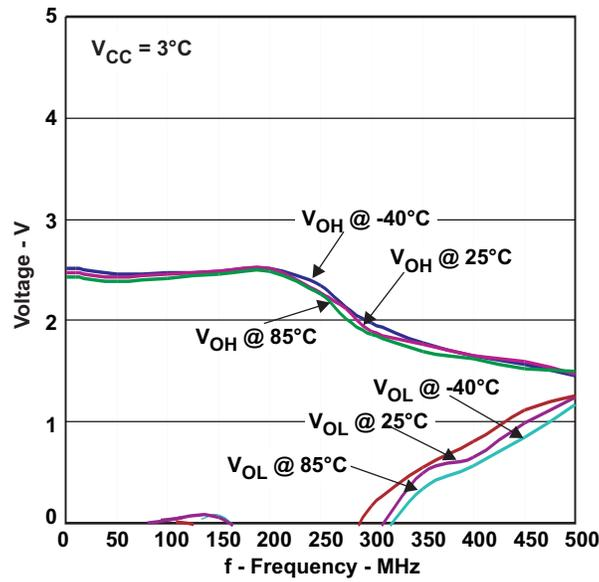
Figure 1. Maximum Switching Frequency  $V_{CC} = 3.0\text{ V}$
