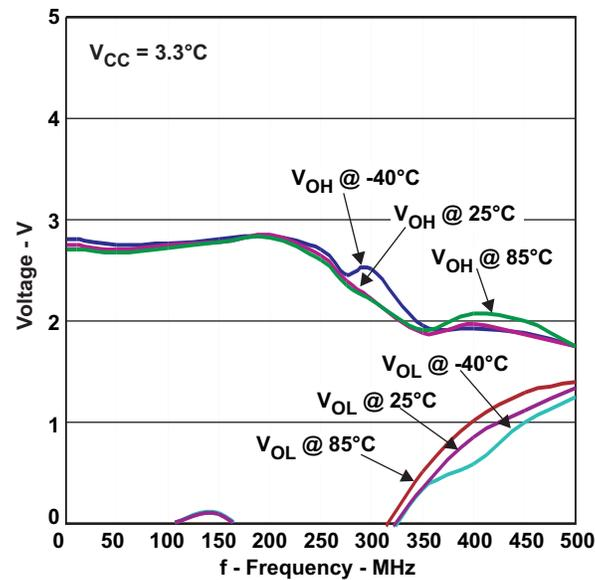
Figure 2. Maximum Switching Frequency  $V_{CC} = 3.3\text{ V}$
