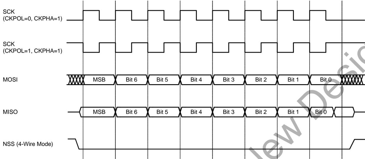
**Figure 24.7. Slave Mode Data/Clock Timing (CKPHA = 1)**
