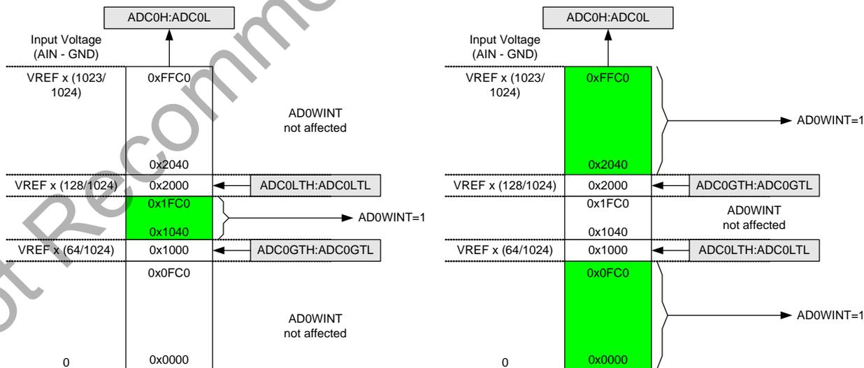
Figure 8.5. ADC Window Compare Example: Left-Justified Data
