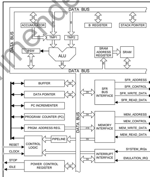
Figure 13.1. CIP-51 Block Diagram
