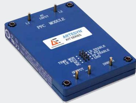
The AIT00ZPFC series of three-quarter-brick power factor correction modules accept a 100–122 Vac input and present a unity power factor. They accommodate AC supply frequencies of 50 Hz, 60 Hz or 360–800 Hz, and a DC input version is also available. Rated at 150 watts, the modules have a high conversion efficiency of 91% and provide a typical output voltage of 393 Vdc.
