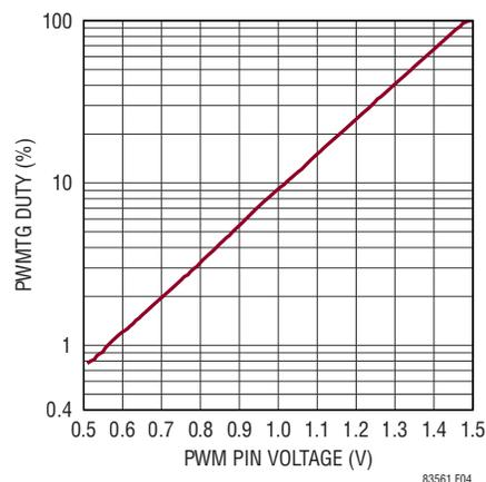
Figure 4. PWM Duty vs PWM Pin Voltages
