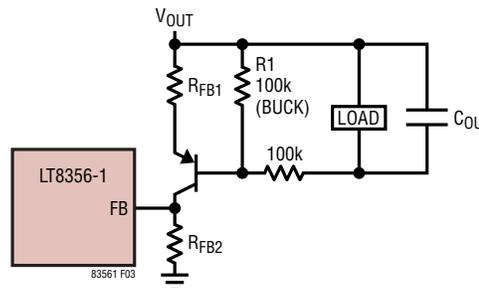
Figure 3. Voltage Feedback Network with Level Shifter
