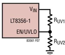
Figure 7. LT8356-1 Resistor Network for Accurate UVLO
