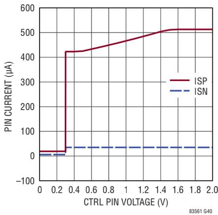
**ISP/ISN Pin Current vs CTRL Voltage at ISN = 0V**
