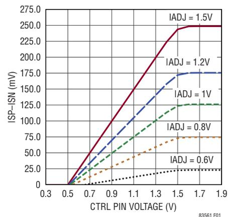
Figure 1.  $V_{ISP}-V_{ISN}$  vs CTRL and  $V_{IADJ}$  Pin Voltage
