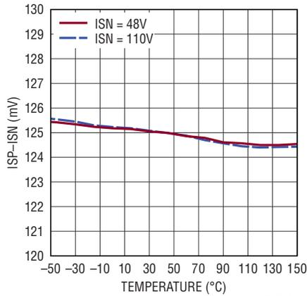
**ISP-ISP Threshold at CTRL = 0.6V vs Temperature**
