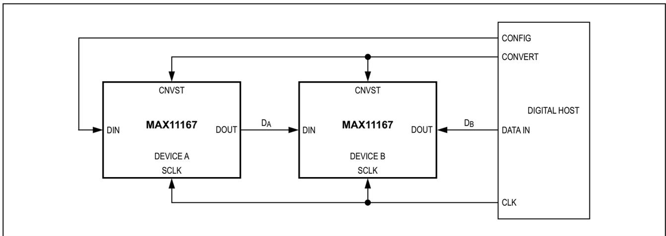
Figure 12. Daisy-Chain, No-Busy Indicator Mode Connection Diagram
