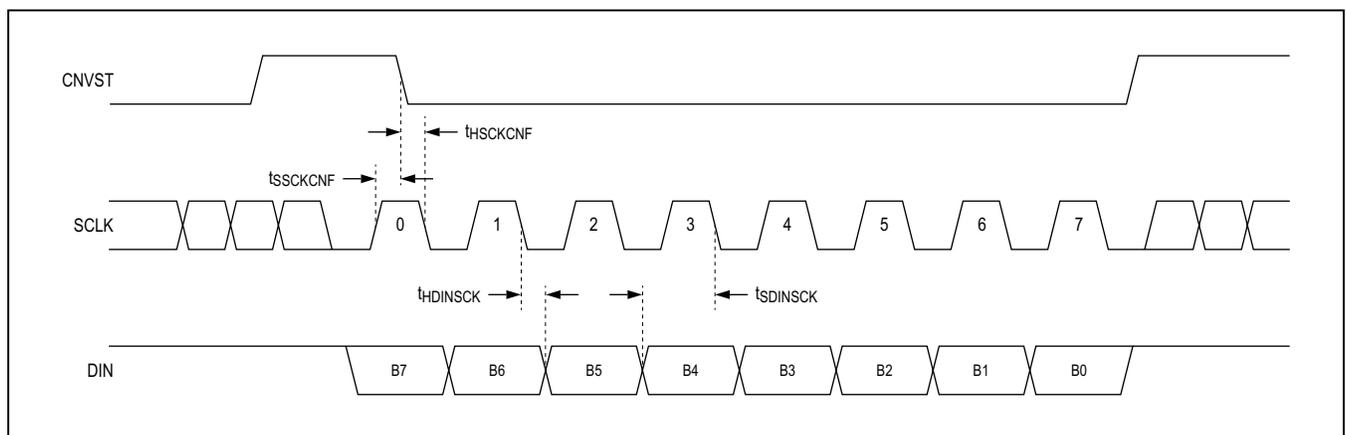
Figure 4. Input Configuration Timing in  $\overline{CS}$  Mode
