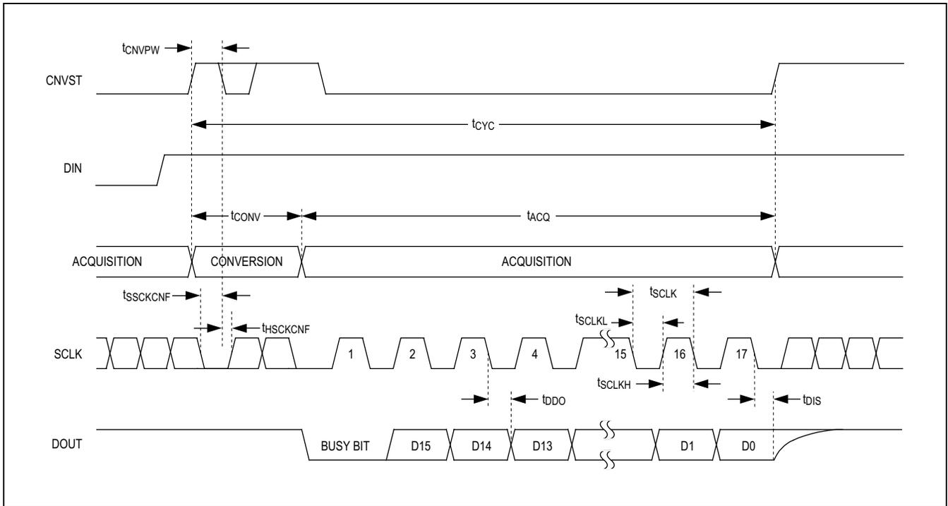
Figure 9.  $\overline{CS}$  With Busy Indicator Mode Timing
