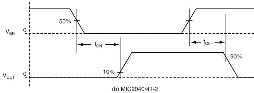
**Figure 1. Turn-On/Turn-Off Delay**
