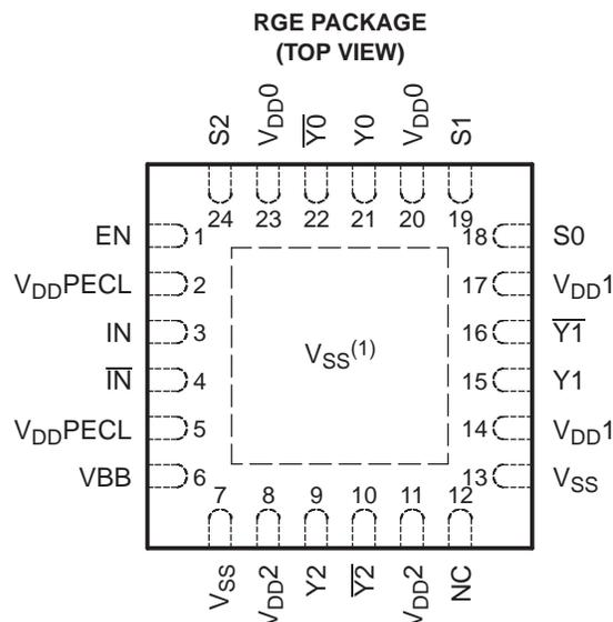
(1) Thermal pad must be connected to  $V_{SS}$ .
