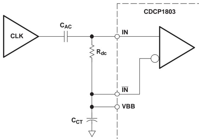
NOTE:  $C_{AC}$  – AC-coupling capacitor (e.g., 10 nF)
