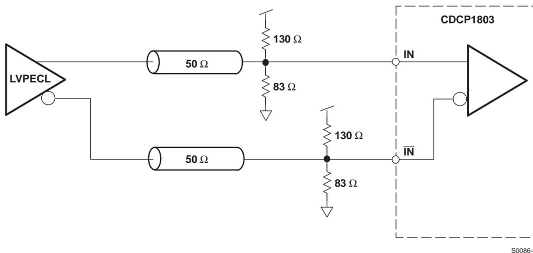
Figure 10. Recommended DC-Coupling LVPECL Receiver Input Termination
