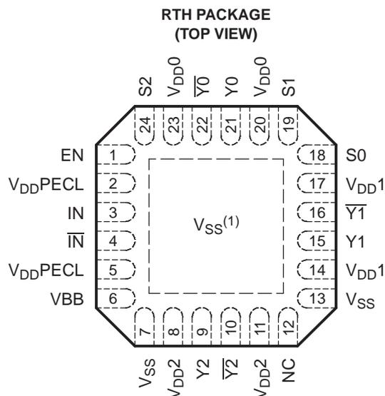
(1) Thermal pad must be connected to  $V_{SS}$ .
