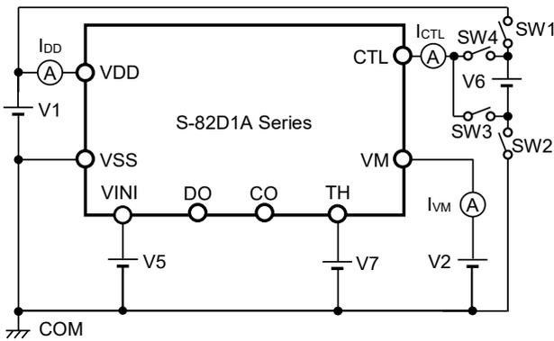
**Figure 5 Test Circuit 3**
