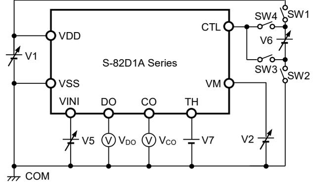
**Figure 4 Test Circuit 2**
