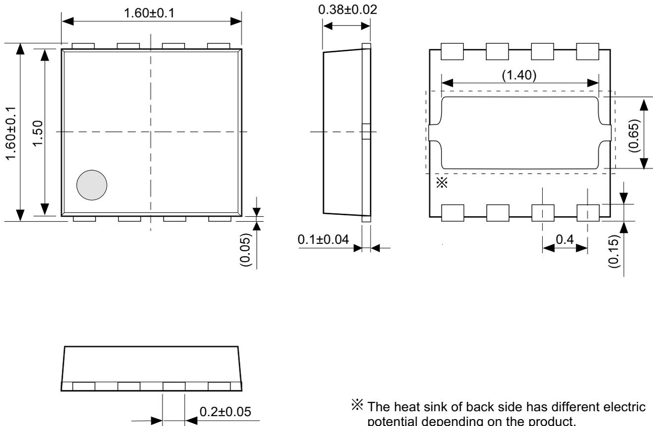
$\times$  The heat sink of back side has different electric potential depending on the product. Confirm specifications of each product. Do not use it as the function of electrode.
