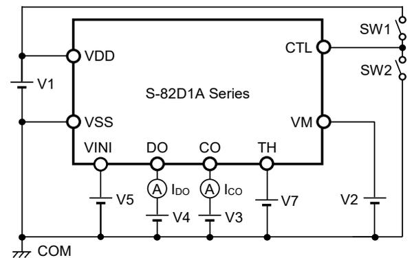
**Figure 6 Test Circuit 4**
