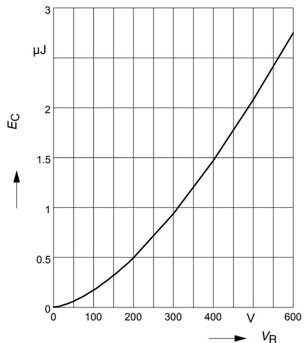
9 Typ. capacitive charge vs. current slope
