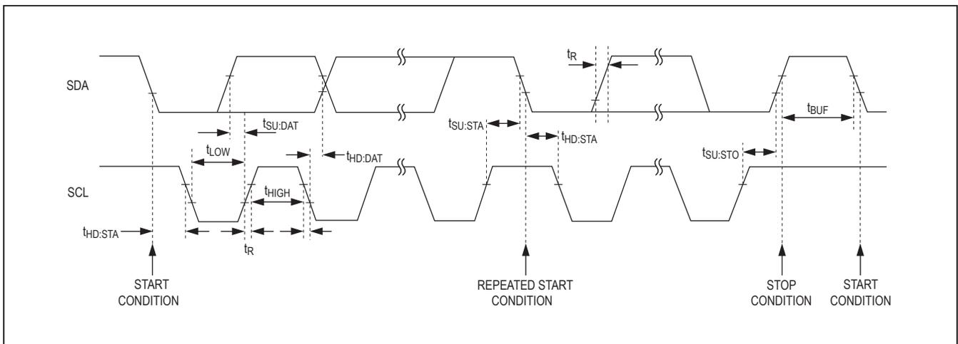
Figure 3. I<sup>2</sup>C Interface Timing Details
