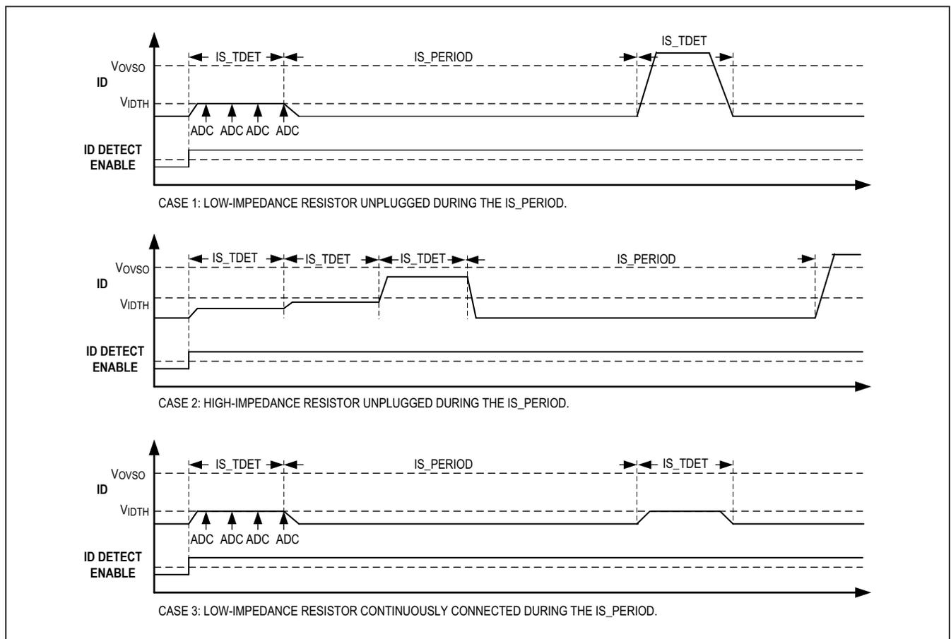
Figure 2. Current Source On-Time Timing Diagram ( $IS\_INIT\_SET = 0$ )
