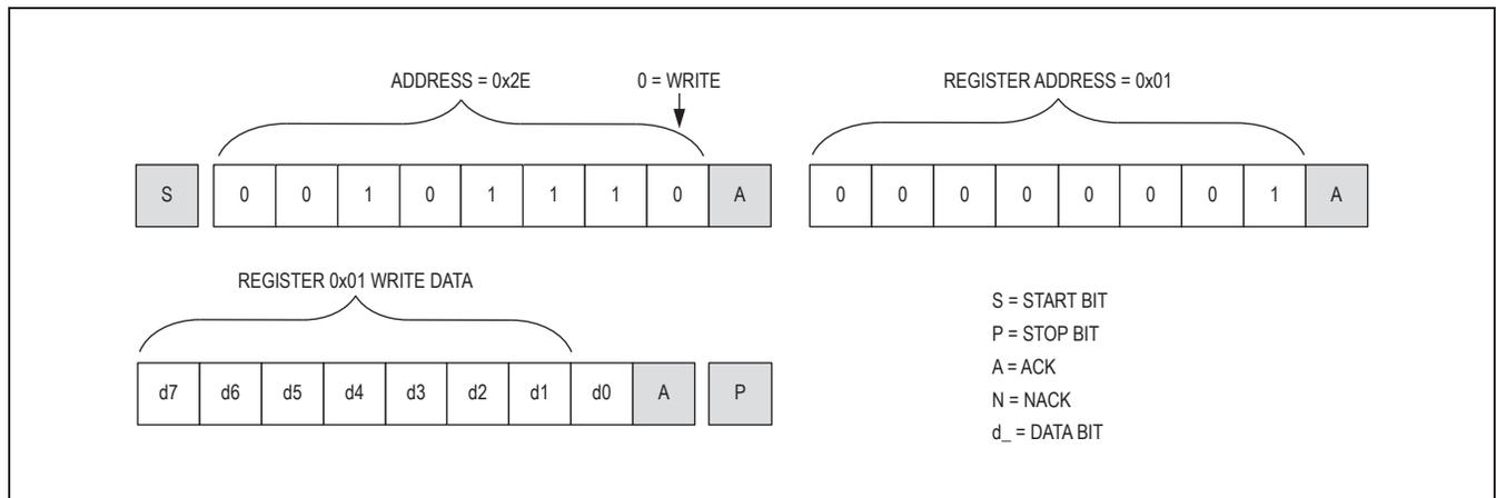
Figure 7. Format for I<sup>2</sup>C Write
