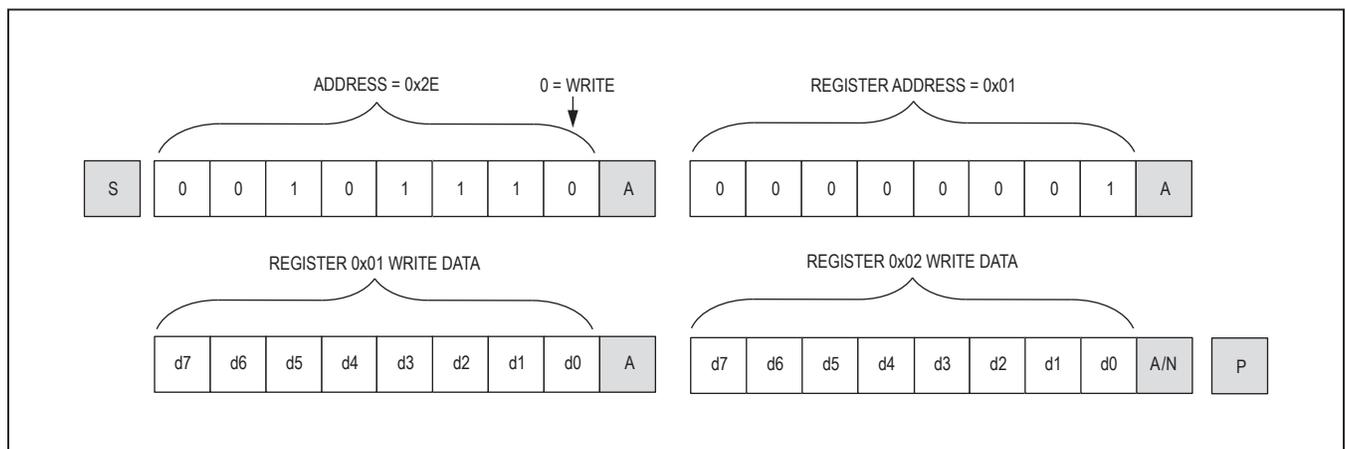
Figure 8. Format for Writing to Multiple Registers
