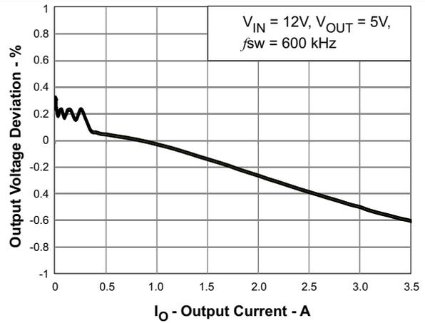
Figure 48. Regulation vs Load Current
