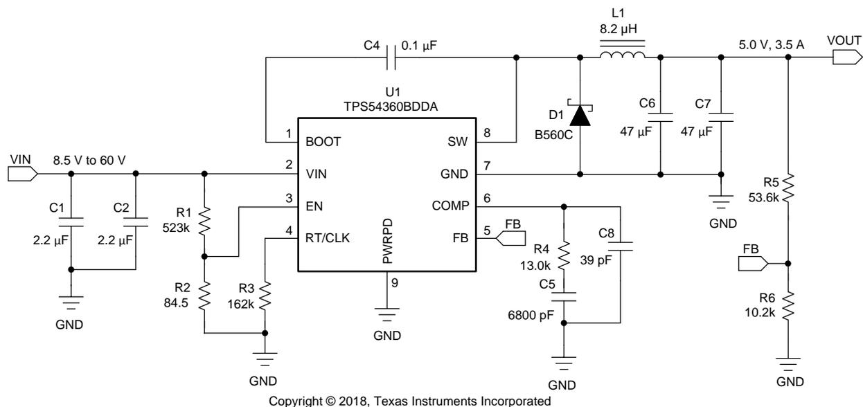
Figure 32. 5 V Output TPS54360B Design Example
