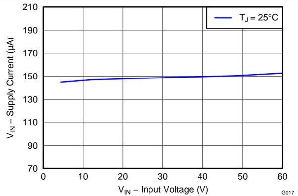
Figure 18. V<sub>IN</sub> Supply Current vs Input Voltage
