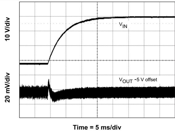
Figure 34. Line Transient (8 V to 40 V)
