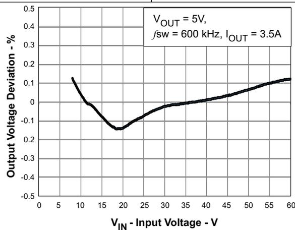
Figure 49. Regulation vs Input Voltage
