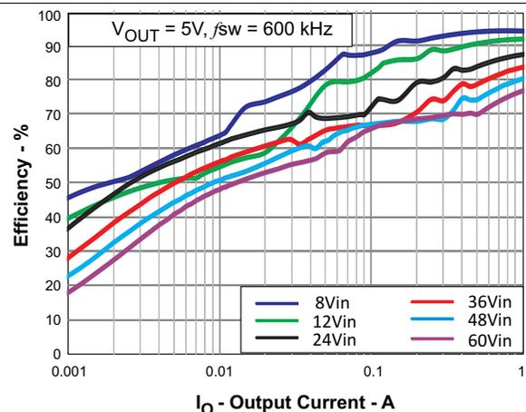
Figure 44. Light Load Efficiency
