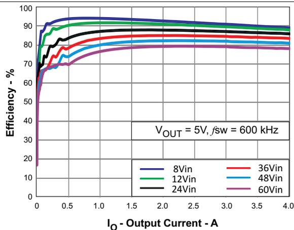
Figure 43. Efficiency vs Load Current
