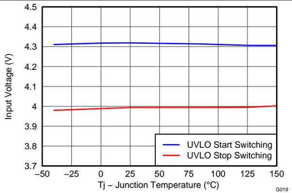
Figure 20. Input Voltage UVLO vs Junction Temperature
