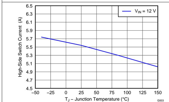
Figure 3. Switch Current Limit vs Junction Temperature
