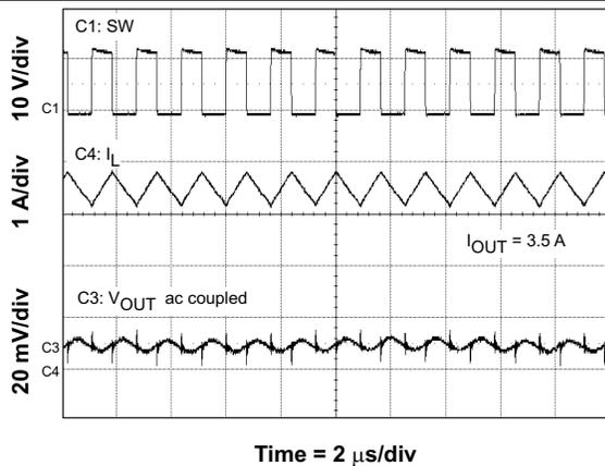
Figure 37. Output Ripple CCM
