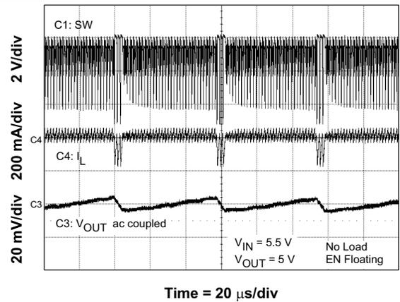
Figure 42. Low Dropout Operation
