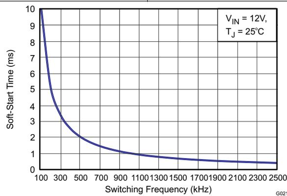
Figure 21. Soft-Start Time vs Switching Frequency
