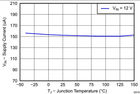
Figure 17. V<sub>IN</sub> Supply Current vs Junction Temperature
