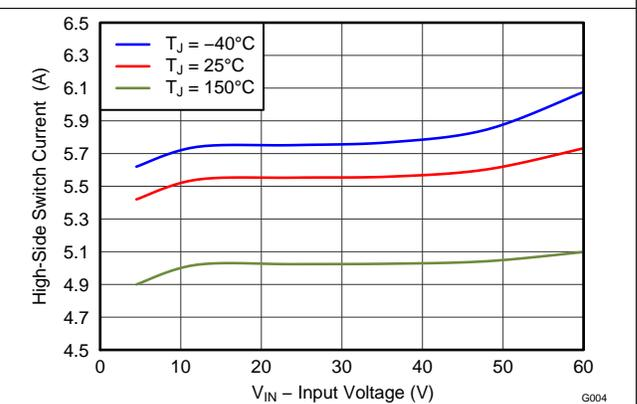
Figure 4. Switch Current Limit vs Input Voltage
