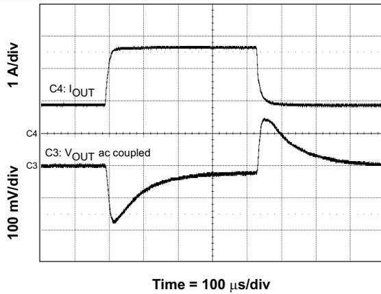
Figure 33. Load Transient
