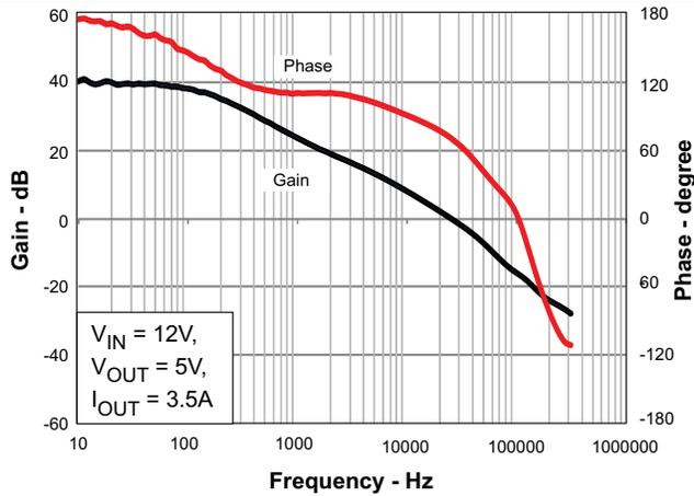
Figure 47. Overall Loop Frequency Response
