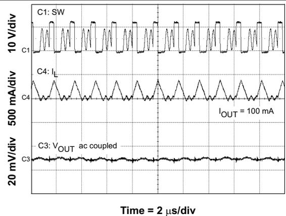
Figure 38. Output Ripple DCM
