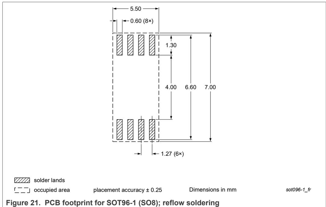
Figure 21. PCB footprint for SOT96-1 (SO8); reflow soldering
