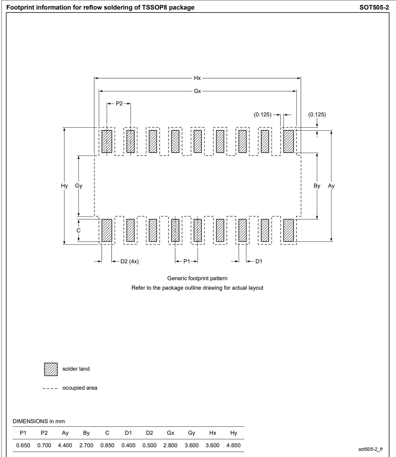
Figure 24. PCB footprint for SOT505-2 (TSSOP8); reflow soldering
