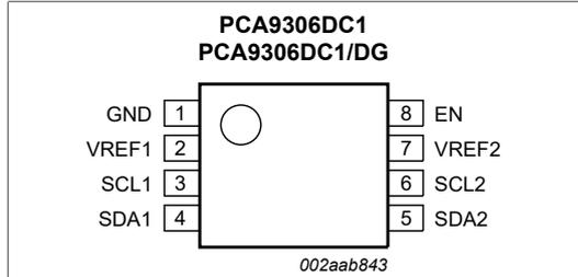
Figure 4. Pin configuration for VSSOP8 (DC1; DC1/DG)
