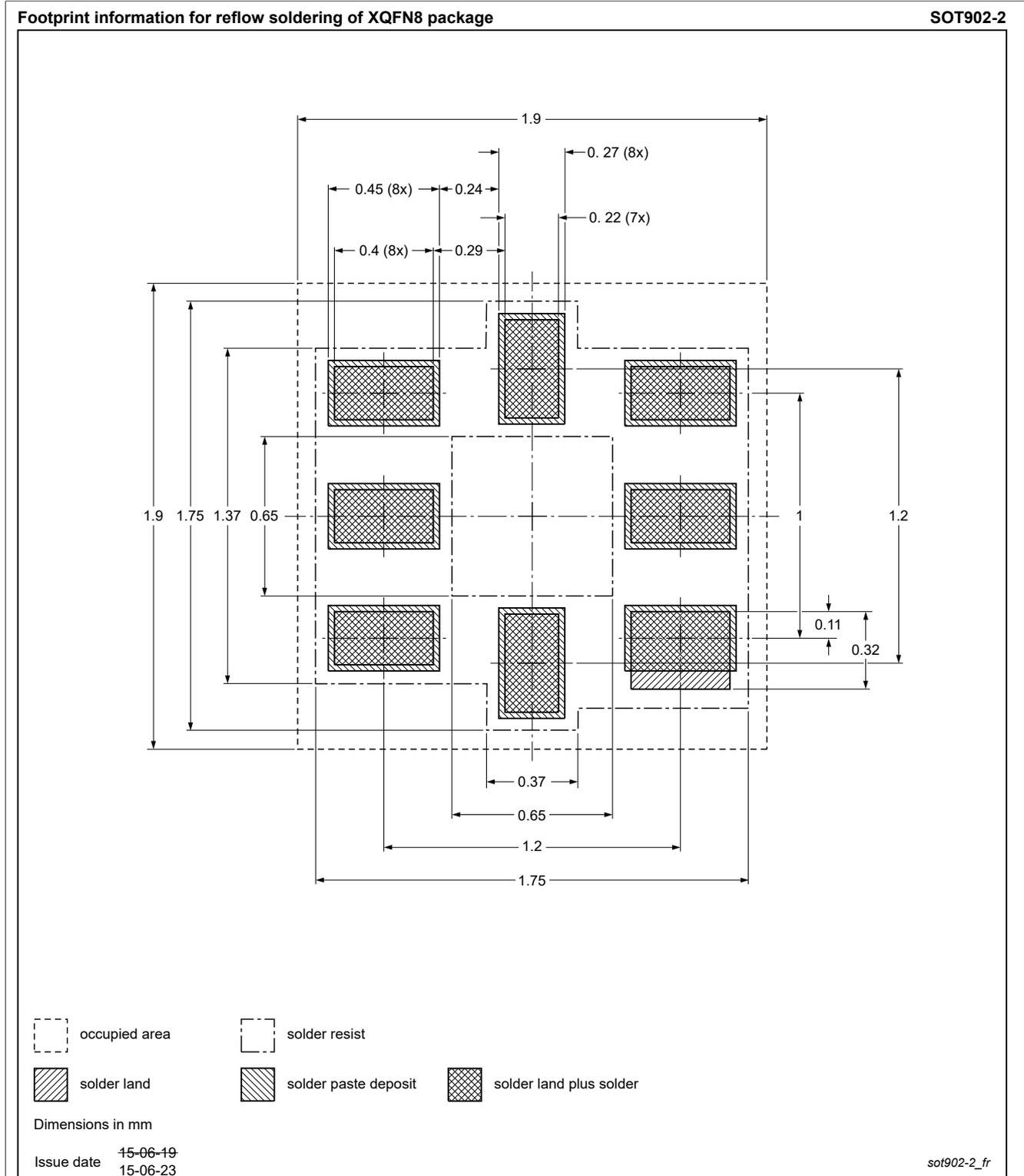
Figure 28. PCB footprint for SOT902-2 (XQFN8); reflow soldering
