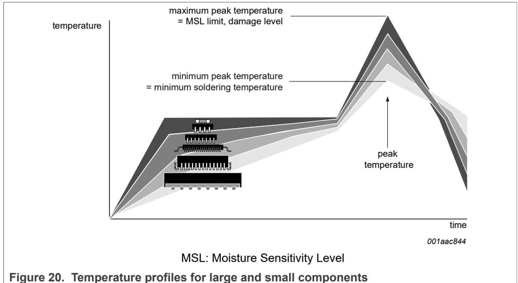
Figure 20. Temperature profiles for large and small components
