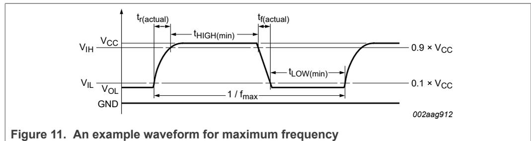
Figure 11. An example waveform for maximum frequency
