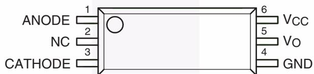
Figure 3. Pin Configuration
