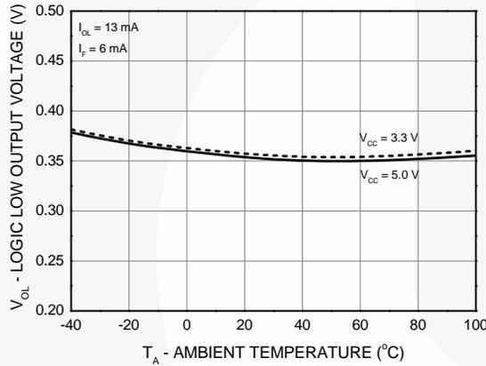
**Figure 6. Logic Low Output Voltage vs. Ambient Temperature**
