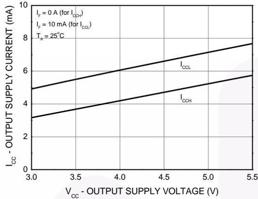
**Figure 10. Output Supply Current vs. Output Supply Voltage**
