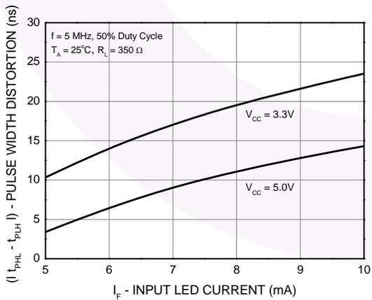
**Figure 14. Pulse Width Distortion vs. Input LED Current**
