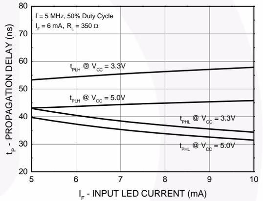
**Figure 13. Propagation Delay vs. Input LED Current**
