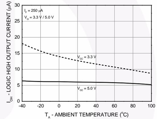
**Figure 7. Logic High Output Current vs. Ambient Temperature**
