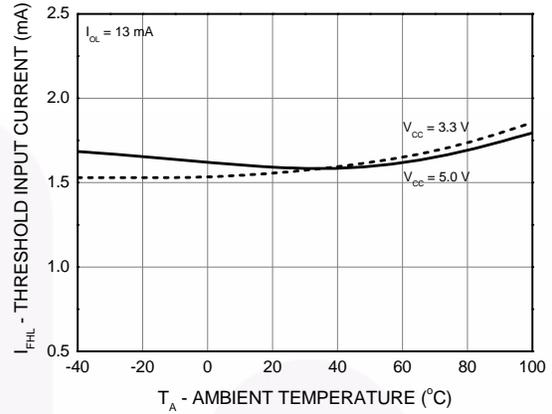
**Figure 5. Threshold Input Current vs. Ambient Temperature**
