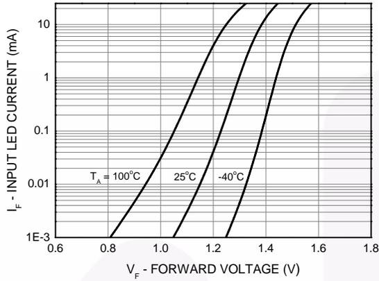
**Figure 4. Input LED Current vs. Forward Voltage**
