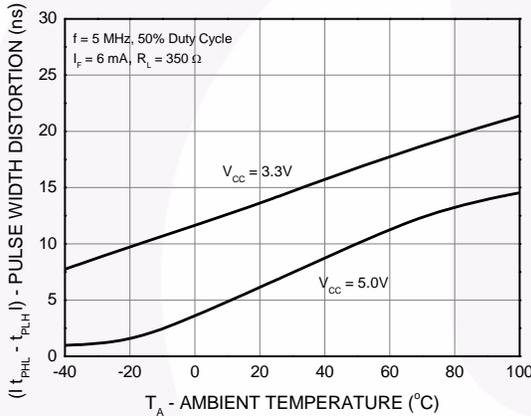
**Figure 12. Pulse Width Distortion vs. Ambient Temperature**
