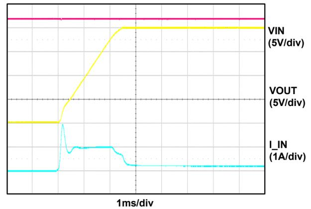
Figure 6. Soft Start Ramp (VIN = 20V)
