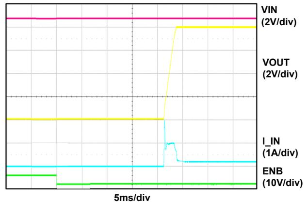
Figure 4. Soft Start Delay Times (VIN = 20V)
