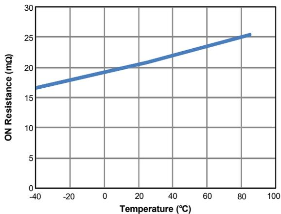
**Figure 19. On Resistance vs. Temperature**
