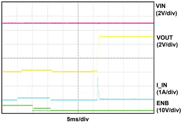
Figure 3. Soft Start Delay Times (VIN = 5V)
