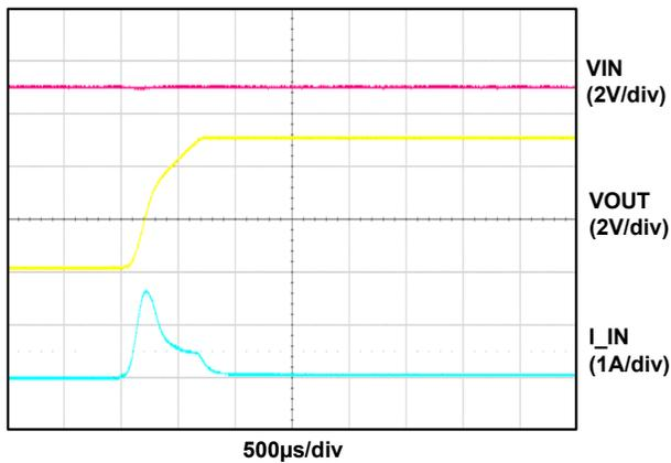
Figure 5. Soft Start Ramp (VIN = 5V)
