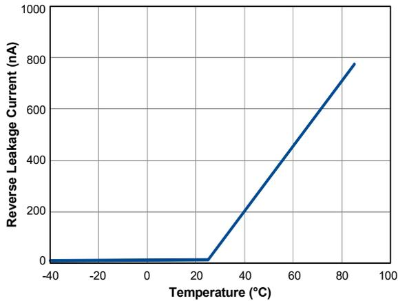
**Figure 17. Reverse Leakage Current vs. Temperature**
