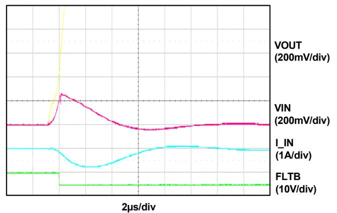
Figure 8. True Reverse Current Blocking (VIN = 5V)
