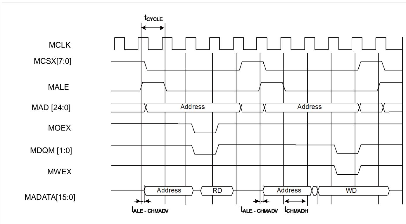
**Multiplexed Bus Access Synchronous SRAM Mode**
