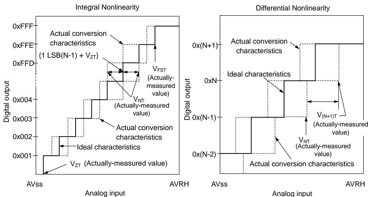
Integral Nonlinearity of digital output N =  $\frac{V_{NT} - \{1\text{LSB} \times (N - 1) + V_{ZT}\}}{1\text{LSB}}$  [LSB]
