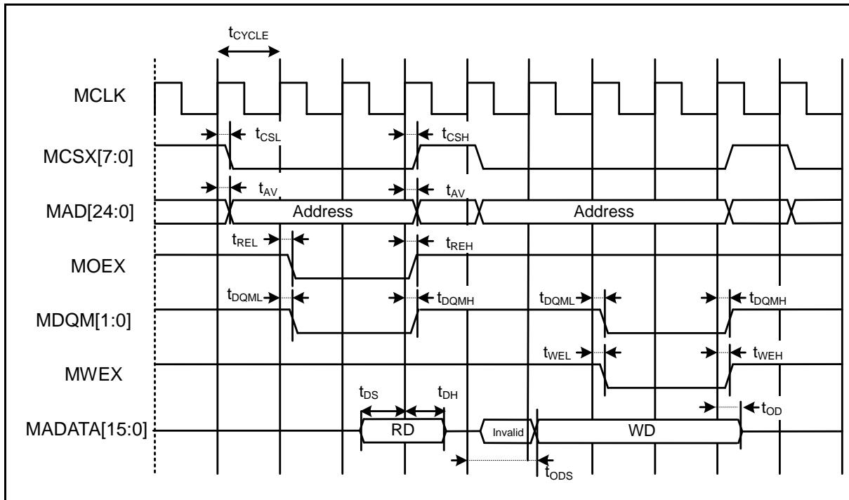
**Multiplexed Bus Access Asynchronous SRAM Mode**
