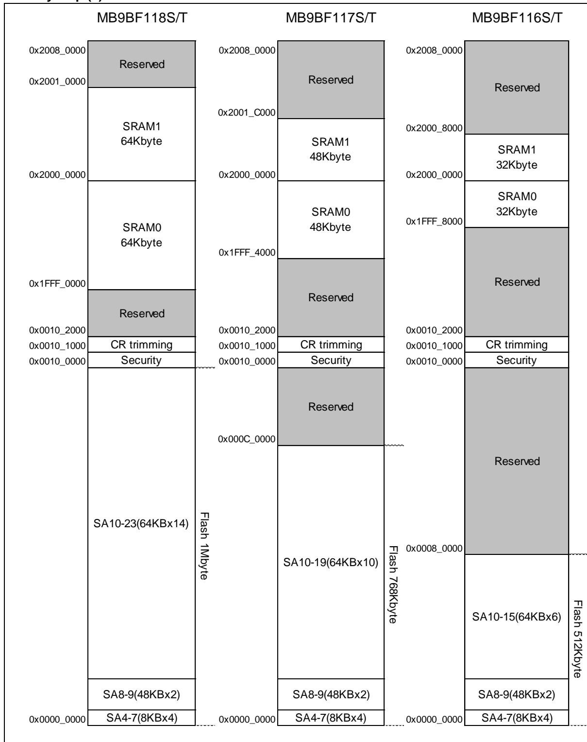
See "MB9BD10T/610T/510T/410T/310T/210T/110T Series Flash programming Manual" for sector structure of Flash.
