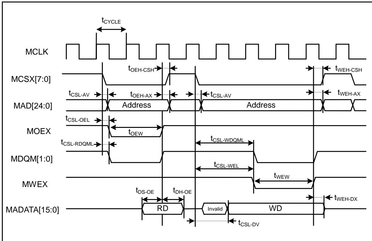
**Separate Bus Access Synchronous SRAM Mode**
