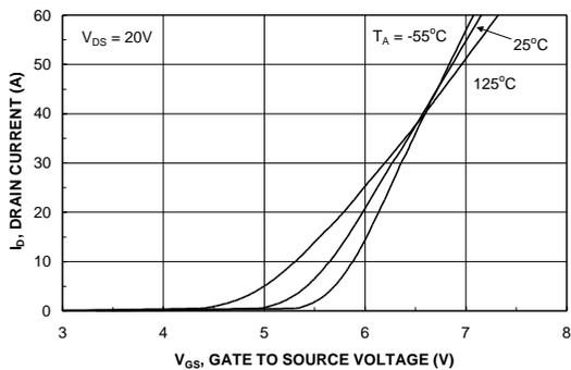
Figure 5. Transfer Characteristics.
