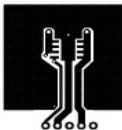
a)  $40^\circ\text{C}/\text{W}$  when mounted on a  $1\text{ in}^2$  pad of 2 oz copper
