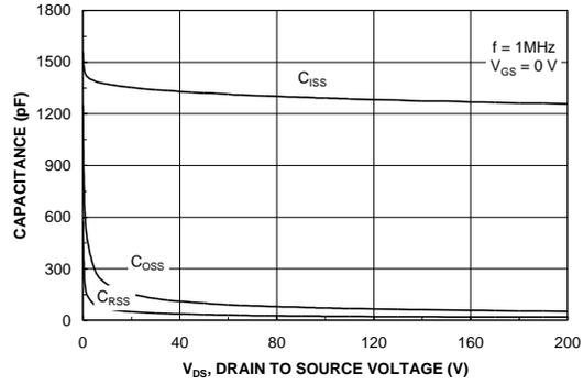
Figure 8. Capacitance Characteristics.
