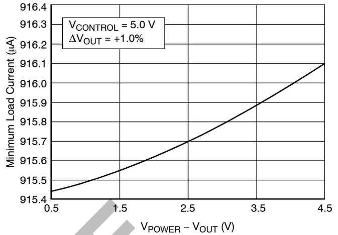
Figure 14. Minimum Load Current vs V<sub>POWER</sub> - V<sub>OUT</sub>
