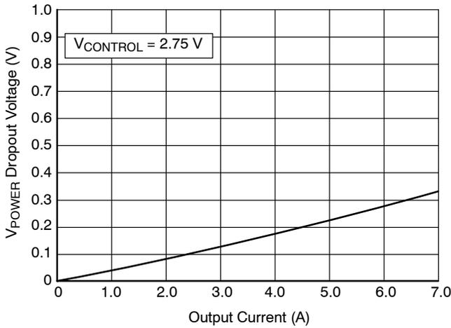
Figure 13. V<sub>POWER</sub> Dropout Voltage vs I<sub>OUT</sub>
