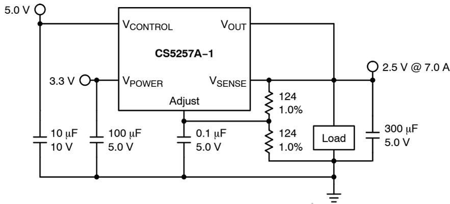
Figure 1. Application Diagram
